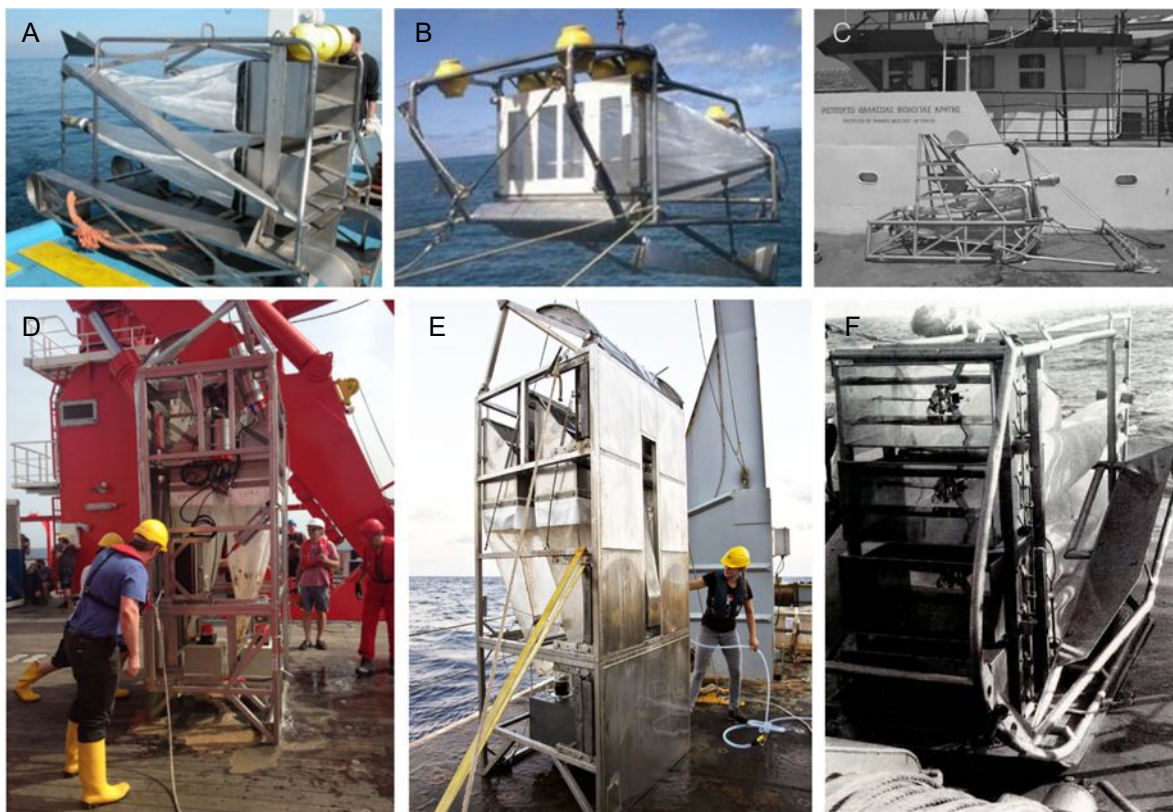
Figure 2.1.1 Examples of gears used to sample the epibenthic/suprabenthic macrofauna. A: Modified Sanders sledge (Mastrototaro et al., 2010); B: Sorbe sledge ( http://www.theseusproject.eu/wiki/Sampling_tools_for_the_marine_environment ); C: TTS sledge (Koulouri et al., 2003); D: EBS sledge ( http://www.oceanblogs.org/so237/2014/12/22/ ); E: Brenke sledge ( http://abyssline.blogspot.pt/2015/03/thats-one-giant-sled-brenke-sledge.html ); F: Macer-Giroq sledge (Dauvin et al., 1995).
