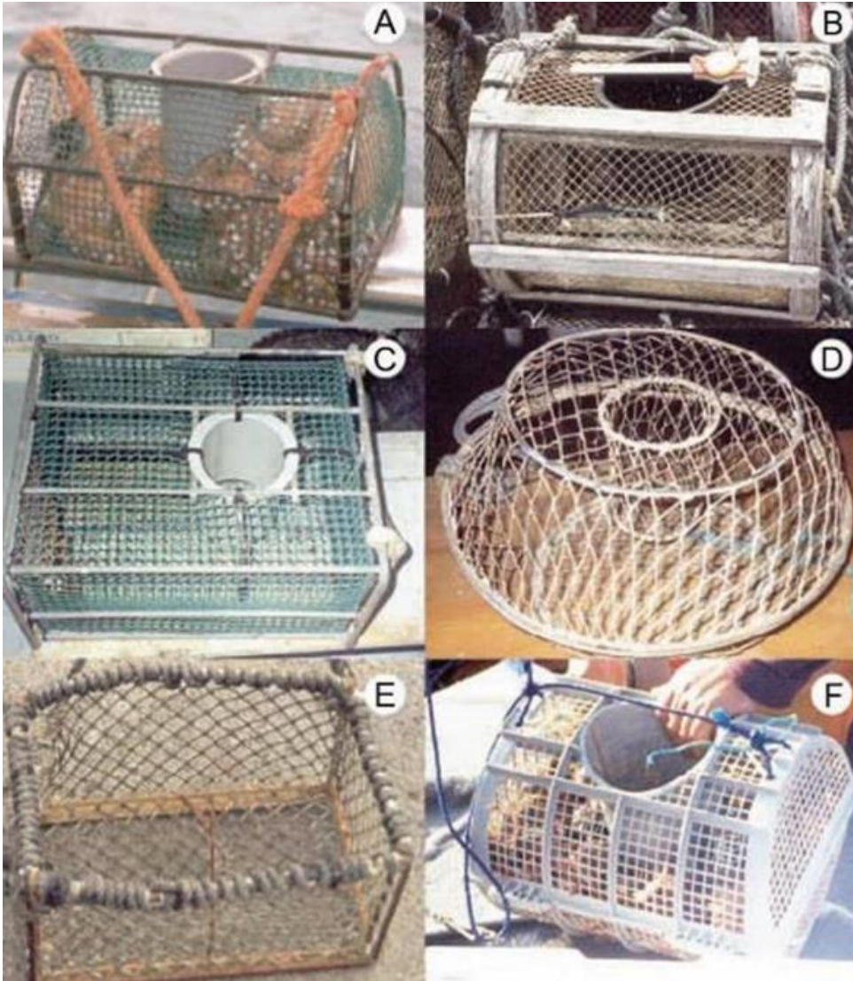
Figure 2. Models of Octopus vulgaris traps used in Galicia, NE Atlantic, made with different shapes and materials. Hemicylindrical, iron (A); cylindrical, wood (B); prismatic, iron (C); toroidal, iron (D); open, iron (E); and cylindrical, plastic (F). From Bañón et al. (2006).
