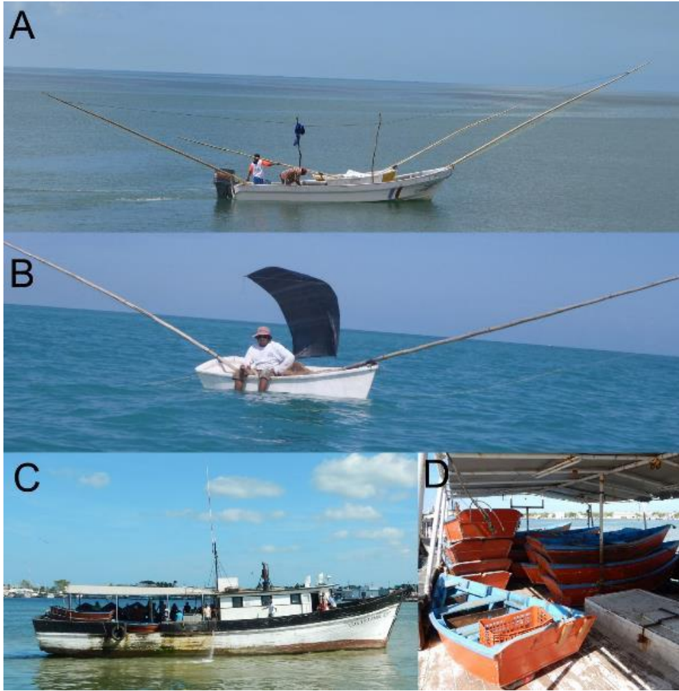
Figure 20. A) An open boat and a dory to Octopus maya fishing grounds. B) A dory (alijo) drifting while fishing for Octopus maya . C) A vessel from the large fleet equipped for fishing octopus. D) Dories piled up in the stern of a vessel.
