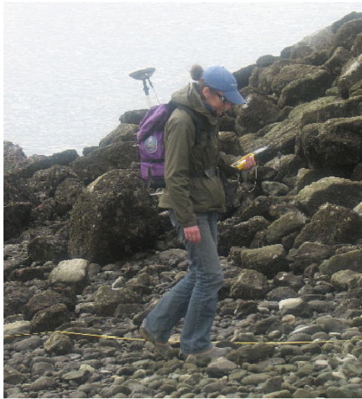
Figure 3a. Beach topography was collected using a Trimble R3 GPS receiver and an L1 antenna. Data was collected by walking along transect lines in the North-South and East-West directions. This grid provided a data density of \sim 2 pts/m 2 .
