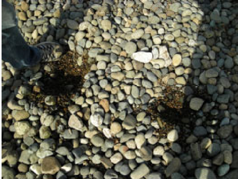
Figure 4. Sediment samples were taken seasonally along the two beach survey transects (BS and BN). Samples were collected from the upper 5 cm where changes in size and sorting and/or changes in topographic features were observed. Subsurface samples were taken where the sediment below the surface clearly differed in size from the surface layer (as seen here).
