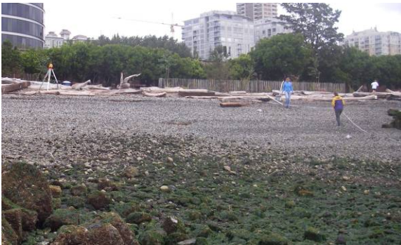
Figure 2b. Beach profile measurements were obtained between a landward endpoint location (i.e., a nail on the sidewalk) to a seaward endpoint location (i.e., a marker on the top of the riprap at the seaward side of the central bench).
