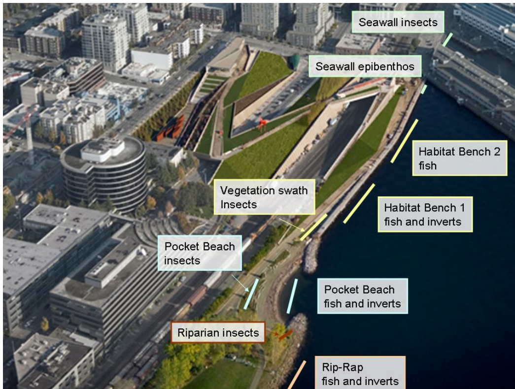
Figure 4. Aerial view of the Olympic Sculpture Park site after construction, showing main fish and invertebrate sampling locations.
