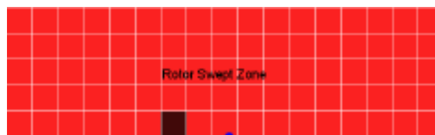
Figure 11: Array of discrete pathways in the rotor swept zone with one of all the Discrete Pathways blocked by a wind turbine
