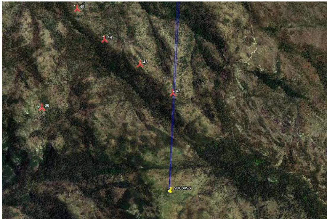
Figure 7: 2 nd Fresnel Zone of links between 9006996 and 440803
