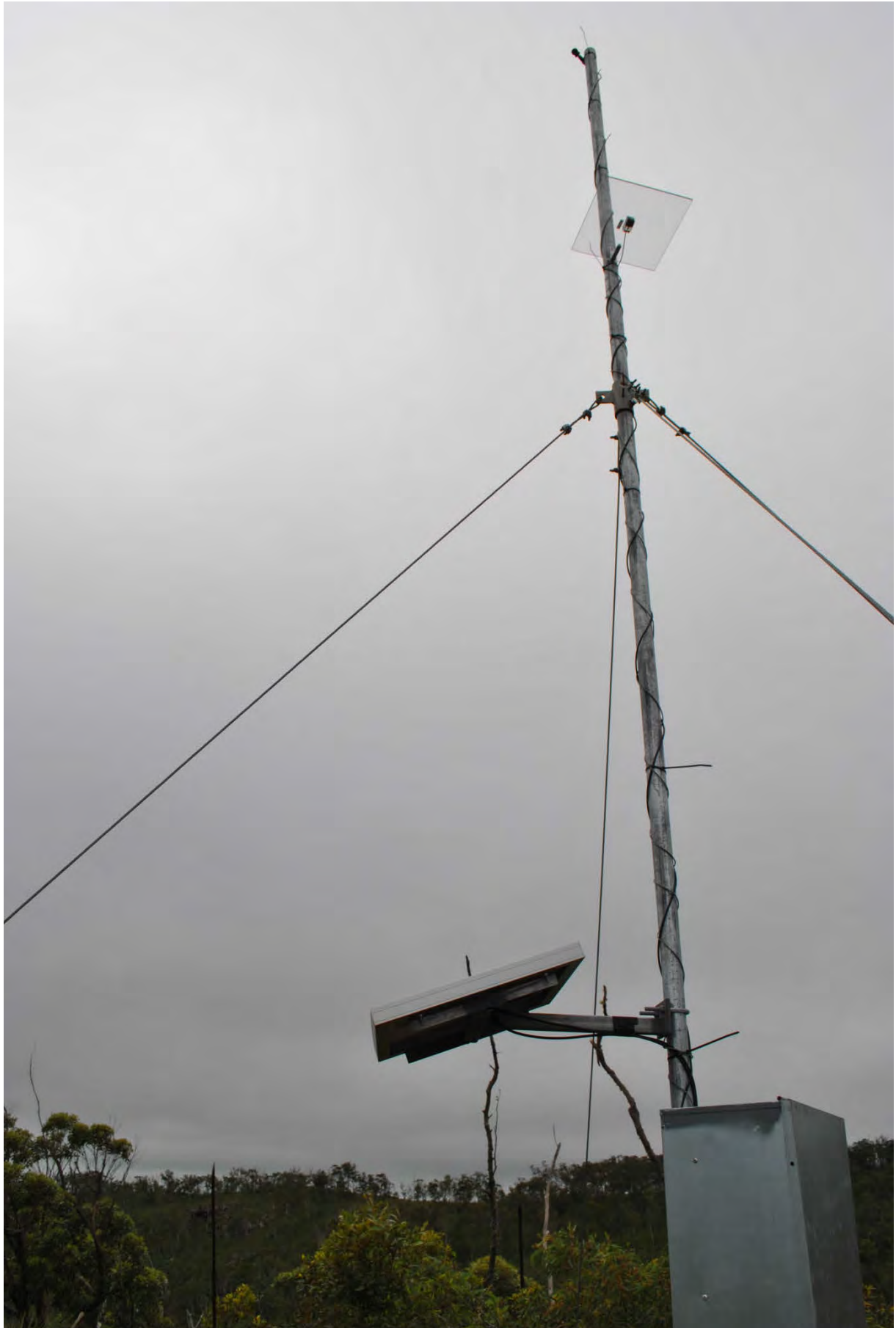
Plate 1 Bat Call Detection Tower (ultrasonic microphone shown at top of pole)
