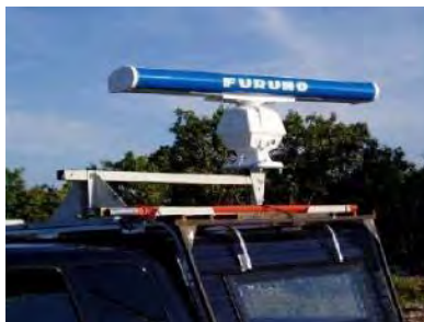
Figure 3: T-bar type marine radar in horizontal surveillance scanning position
