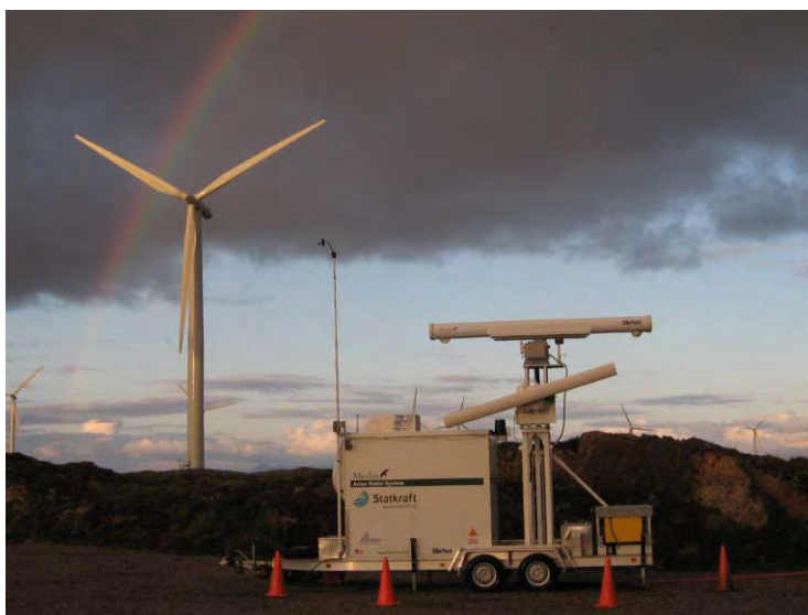
Figure 1: MERLIN Avian Radar System at Smola Wind Park, Norway (Owner: Staatkraft)
