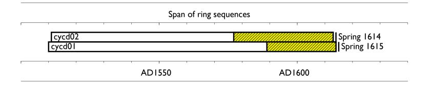
**Figure 2:** Bar diagram showing the relative positions of overlap of the dated samples, with their actual or likely felling dates / date ranges. White sections represent heartwood rings and yellow hatched sections represent sapwood, narrow bars represent additional unmeasured rings.
