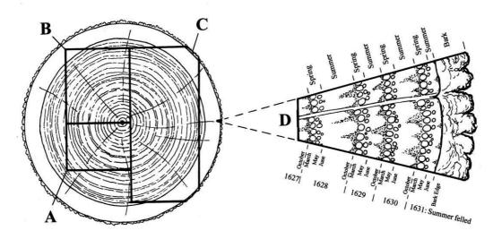
Section of tree with conversion methods showing three types of sapwood retention resulting in A *terminus post quem*, B a felling date range, and C a precise felling date. Enlarged area D shows the outermost rings of the sapwood with growing seasons (Miles 1997, 42)
