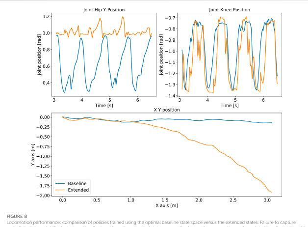
periodicity (top) and drift of robot position (bottom) from the extended state space policy (orange), compared to our formulated baseline policy with optimal state space (blue).
