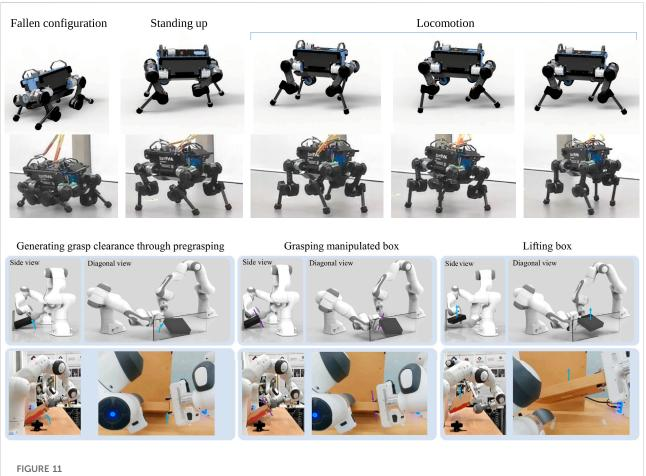
Multi-expert policies in simulation and on the real robot. Top: Robust locomotion of gait recovery from a prone position and smooth transitions to trotting. Bottom: Dual-arm cooperative manipulation and grasping.
