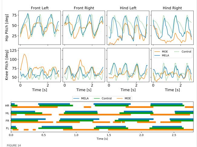
Locomotion comparison between control, MoE and MELA. Top: Joint position. Bottom: Gait pattern of Front Left (FL), Front Right (FR), Hind Left (HL), Hind Right (HR) feet.
