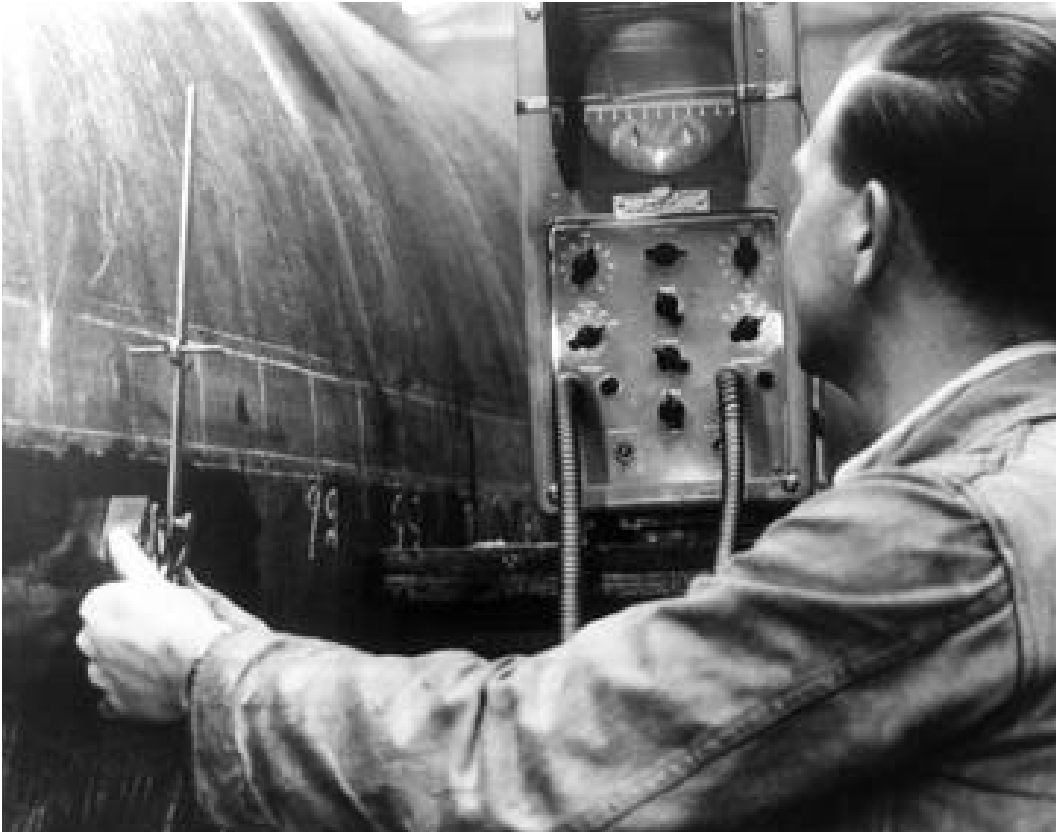
Figure 3. A Kelvin & Hughes Mark IV flaw detector being used by the late Mr J Davis in the Babcock and Wilcox factory at Renfrew, where Ian Donald did his very earliest investigations on biological materials.
