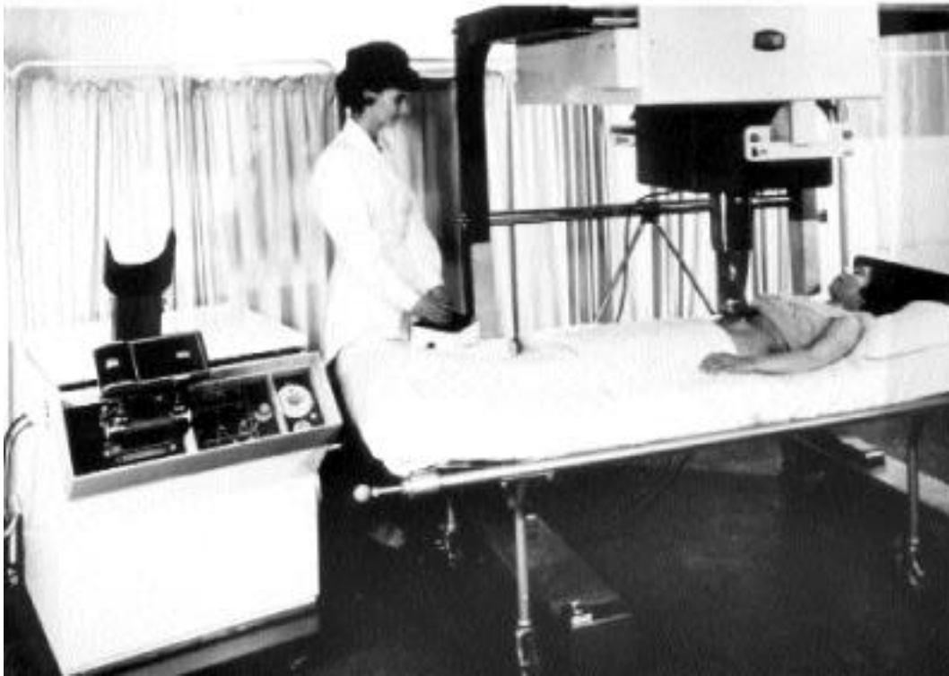
Figure 13. The Disonograph was modular in design and construction. Shown here, on the left of the photograph, is the electronics console which formed the lower half of the machine. The mechanical assembly on the right is the automatic scanner. This was originally used with the electronics assembly designed for the 'bed-table scanner'; at a later date this was replaced by a Disonograph electronics console as seen here. This photograph was taken in the factory at Hillington, Glasgow, c. 1966.
