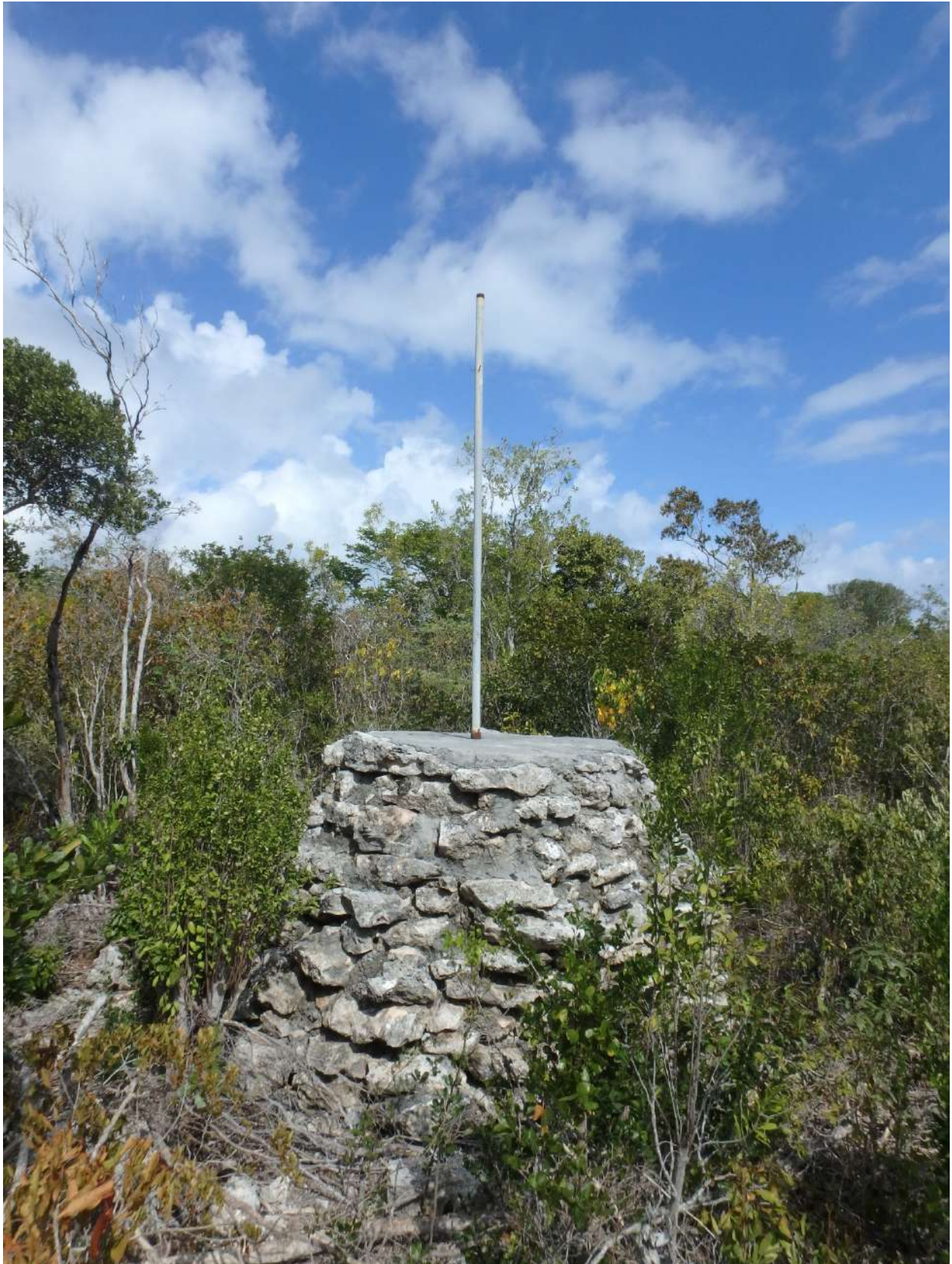
Surveyor's Cairn along North Property Line at North 24 degrees 38 min 17.5 sec - West 076 Degrees 01min 22.3sec
