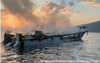
interconnected smoke-detectors in all passenger areas. It also recommends that the primary and secondary means of escape should lead into separate spaces.
