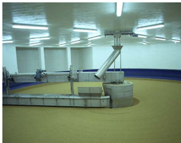
Sophus Fuglsang Export-Maltfabrik in Haderslev and Thisted produce in total approximately 150,000 tons of malt a year. With this amount of malt about 3 billion bottles of beer can be brewed. The photo shows one of the malt kilns in Thisted. Photo: Fuglsang
