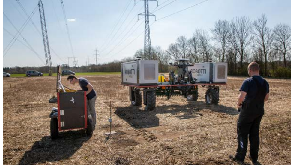
Weeding machine robot developed to weed crops such as sugar beets and other row crops - with a great potential to reduce herbicide spraying
