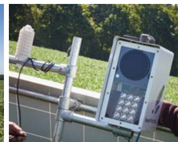
Part of one of the advanced cameras that photographs and registers all insects that move around in its zone of operation
