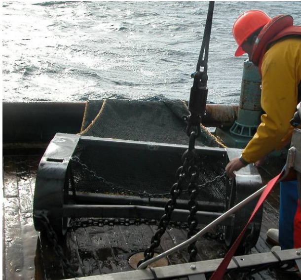
Figure 9: Epibenthic dredge used during voyage to sample epibenthos.
