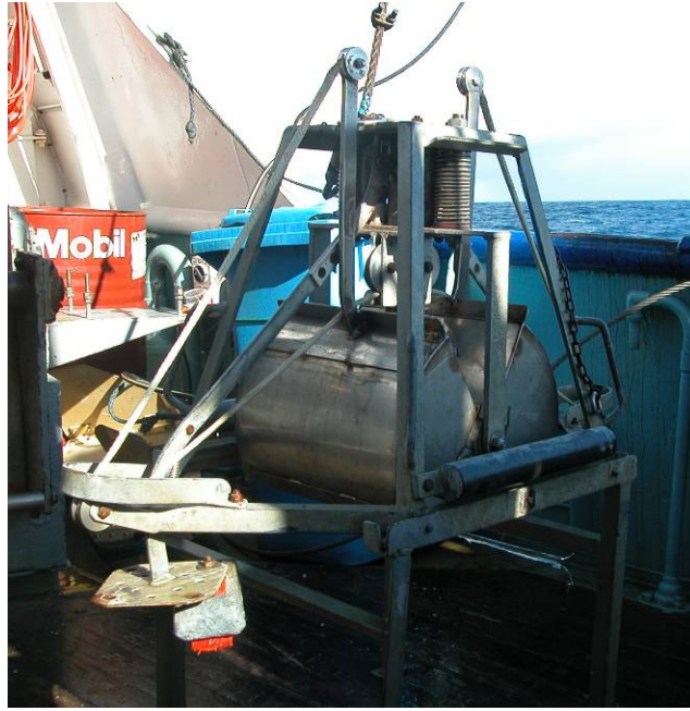
Figure 11: Smith-McIntyre grab used during survey to collect sediment and infaunal material.
