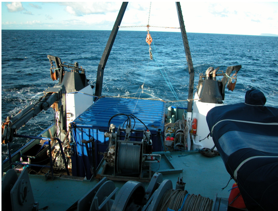
Figure 3: Side-scan sonar winch (in front of blue container) with side-scan sonar cable deployed through block over stern of vessel.
