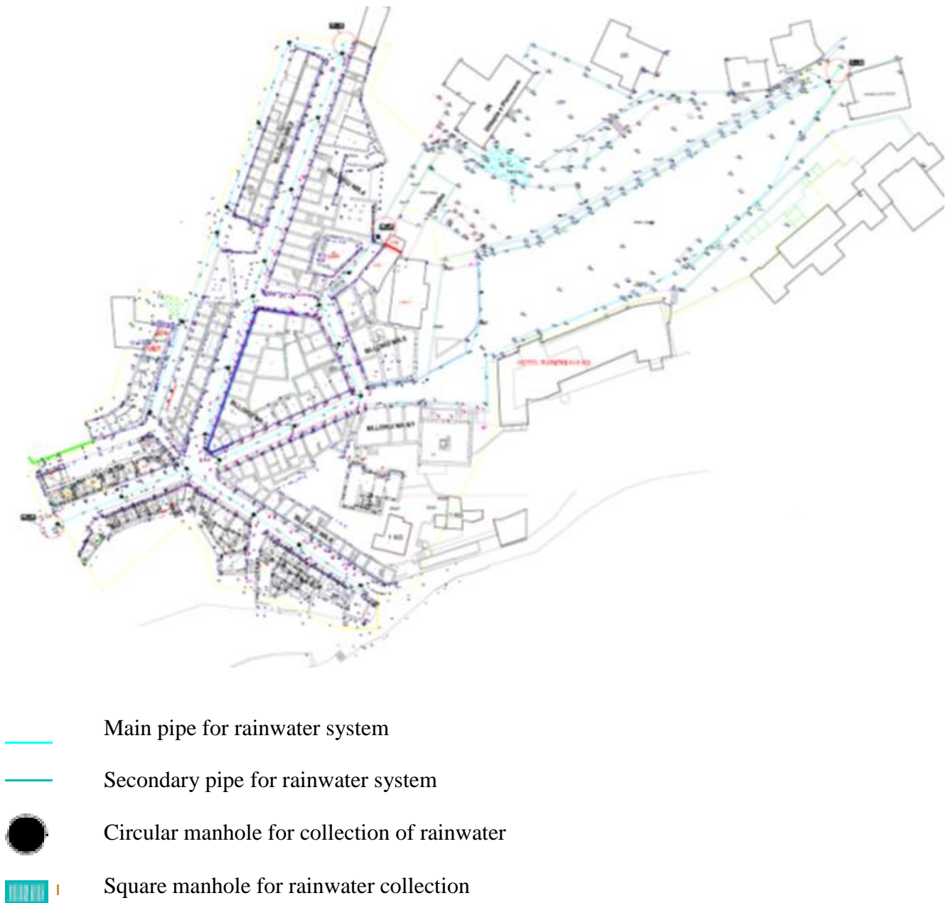
Figure 18: The layout of rainwater discharge system
