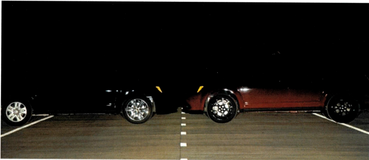
Figure 2 - Photograph of Subjective Evaluation using Jeep Cherokee Low Beam Headlamps as light source. Camera lens set at centerline of road, centerline of the Jeep Cherokee, and height above ground equivalent to that of an average height female driver sitting in the driver's seat of the Jeep Cherokee.
