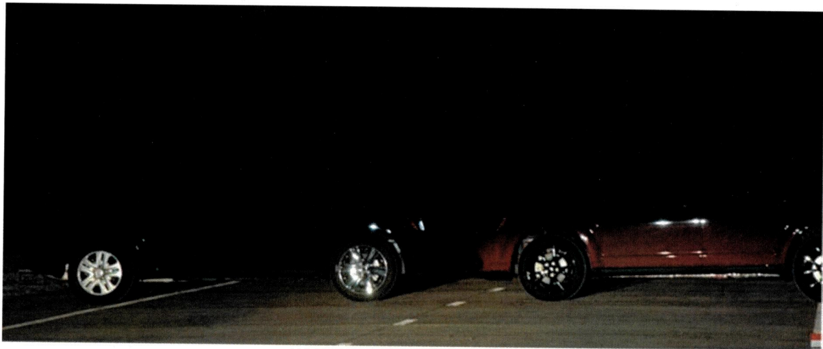
Figure 8 - Photograph of Subjective Evaluation using Jeep Cherokee Low Beam Headlamps as source of illumination. Camera lens set at right edge of pavement, centerline of the Jeep Cherokee, and height above ground equivalent to that of an average height female driver.
