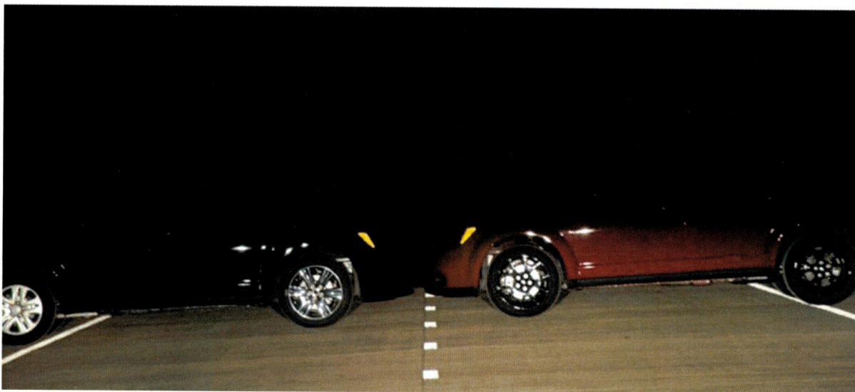
Figure 10- Photograph of Subjective Evaluation using Ram 1500 Pickup Truck Low Beam Headlamps as source of illumination. Camera lens set at right edge of pavement, centerline of Ram 1500 Pickup Truck, and height above ground equivalent to that of an average height female driver sitting in the driver's seat of the Ram 1500 Pickup Truck.
