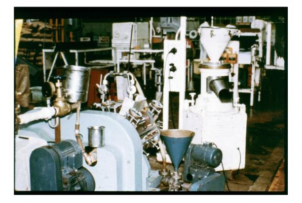
In the foreground is a rotary drum dryer chosen for surface drying of emulsified food mixes. At the rear is a grinder that can handle the mixes, even emulsifying fish bones.
