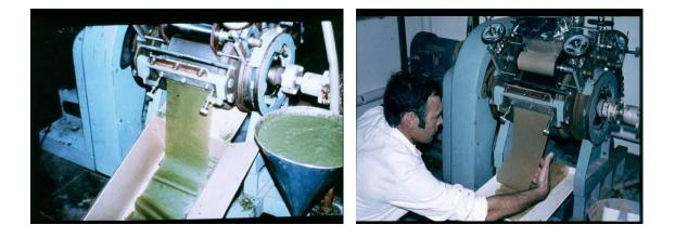
The food pastes were poured into the funnel and from there pumped at a controlled rate onto the steamheated roller drier. This flashcooked the proteins to give a paperlike texture, just as occurred with the frying pan and wallpaper roller trials. The vegetable and meaty mixes are shown.
