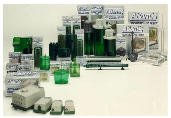
There were some novel features – working with consultant engineers, David made the airpumps the most silent on the market by including a 'tuned' input tube to the diaphragm oscillator. The heaters had silver sand included to make the 'glowing' heating elements invisible. This also spread the heat to give a more uniform temperature profile with consequent higher efficiency and much longer life (Atlantis heaterstats are still in continuous use 20 years later).
