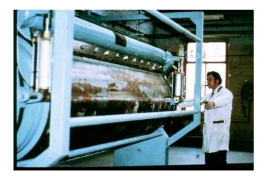
Here is the commercial version of the rotary drum dryer at Pedigree Petfoods being installed at the Thomas's factory at Shelf, near Halifax, West Yorkshire. Delivered in April 1974, this roller is 9 feet long.
