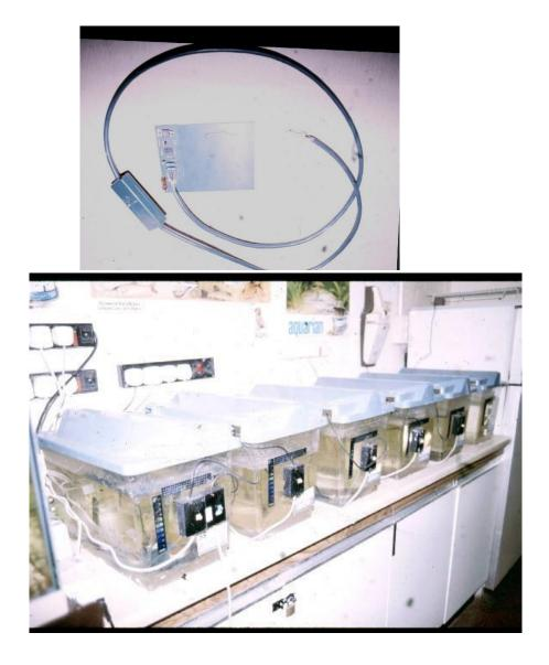
This was a novel heater where a heating element was buried in a flat plastic plate and an electronic control unit, sealed in resin, operated the temperature via an external control box.
