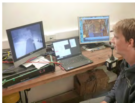
Figure 3. The Benthic Disturber being monitored during operation (the chimney plume is on the left screen)
