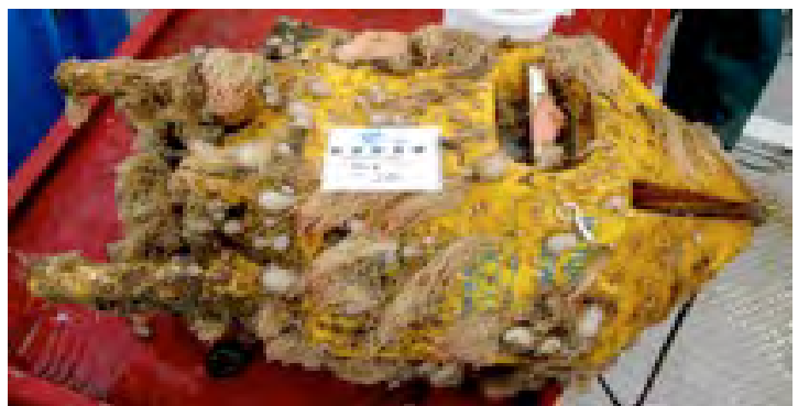
Figure 2. OTN receiver float covered in Vazella sponges, amongst other biofouling (photo: DFO)
