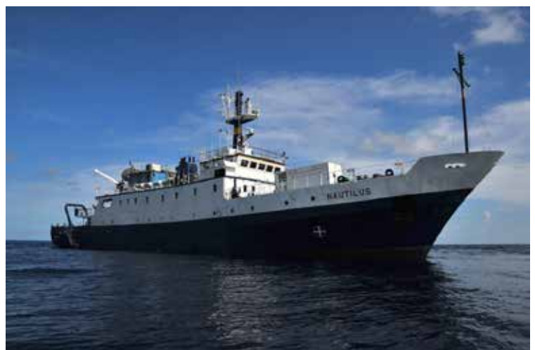
Exploration Vessel Nautilus is a 64-m vessel equipped with satellite telepresence system, dynamic positioning, an EM-302 multibeam echosounder, and the 4,000-m Hercules/Argus remotely operated vehicle (ROV) system. Image courtesy Katy Croff Bell
