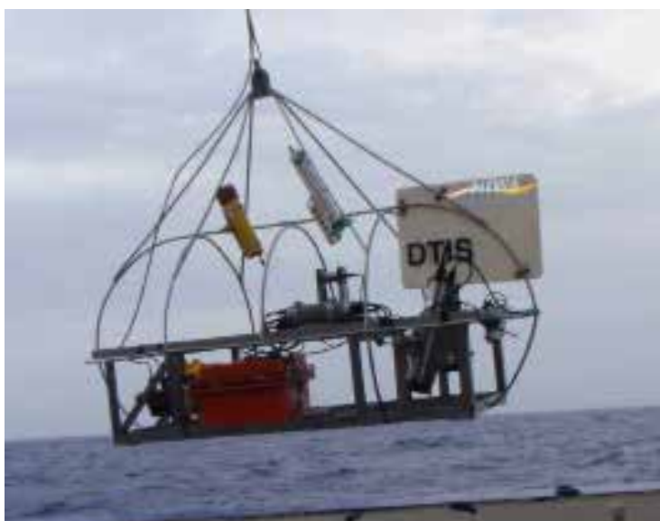
Figure 2: NIWA's Deep towed imaging system (DTIS), which was the main sampling tool used for the survey. Image courtesy Clark & Rowden
