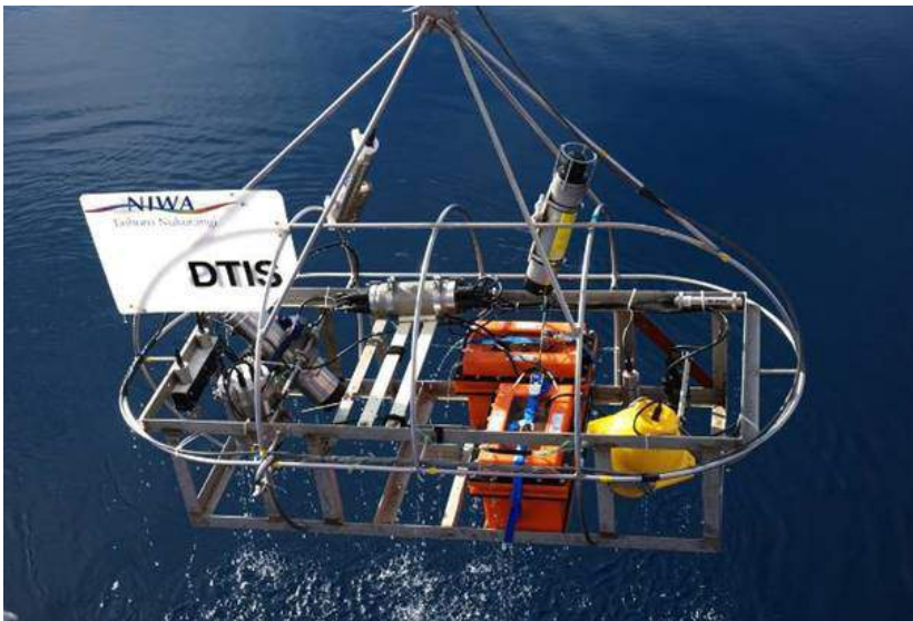
Figure 3: The towed camera system (DTIS) employed during the survey.
