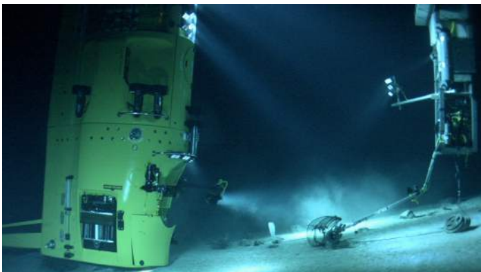
Figure 1: The DEEPSEA CHALLENGE submersible and lander meet up at ~1.1 km depth near the Ulithi atoll. Photo taken by an ROV.
