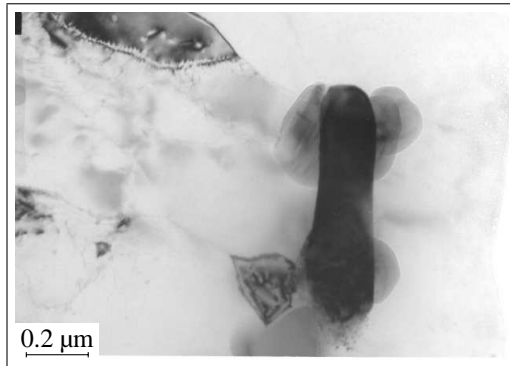
Figure 3.9: Dark \alpha\text{-Al}_{15}(\text{Mn}, \text{Fe})_3\text{Si}_2 particle surrounded by lighter Si particles in LV alloy.
