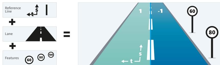
**Figure 2.3:** Elements of road definition from *project OpenDrive* [2].
