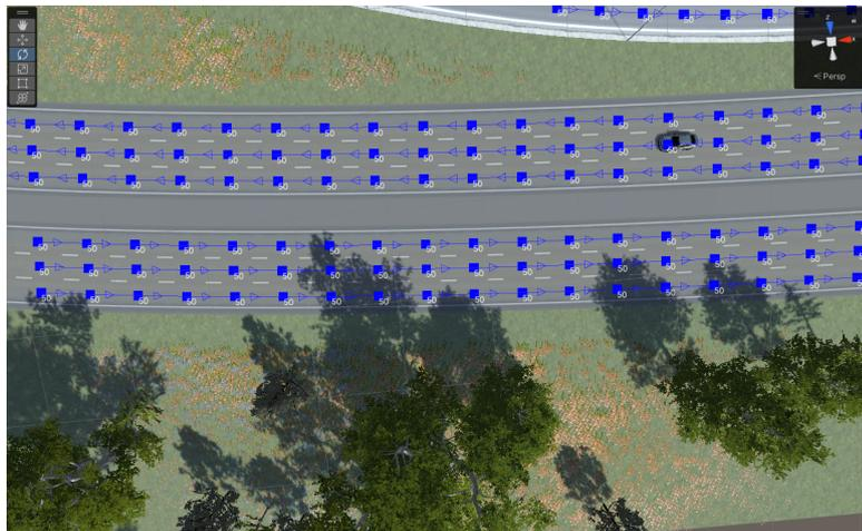
**Figure 2.10:** Nodes generated by traffic system according to EasyRoads by *Mobile Traffic System* [24].
