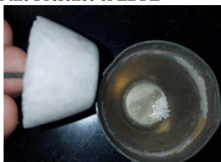
Figure 4-17: Salt (\text{Li}_{0.62}\text{K}_{0.38})_2\text{CO}_3 + 13 mol% LiOH with 8wt% LDPE) with embedded electrode crucible after 90 minute pre-treatment at 600°C in \text{N}_2
