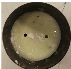
Figure 3-2: Pre-melted and solidified Sodium/Lithium Borate in a nickel crucible prior to experimentation. The green coloration suggests dissolution of nickel oxide into the melt.
