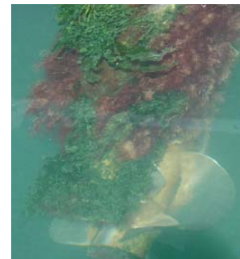
A heavily fouled propeller of a recreational boat that may transport organisms from one location to another. Photo credit: J. Pederson
