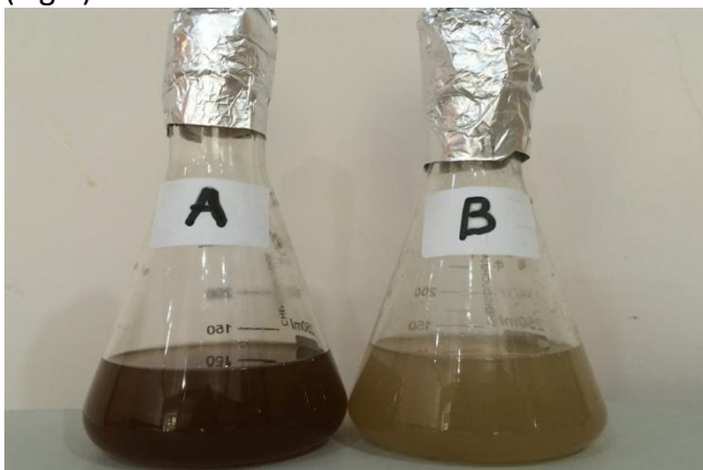
Fig.1. Color change of reaction mixture during formation of silver nanoparticles with the biomass of Actinomyces spp. NSX-333: a-experiment; b-control
