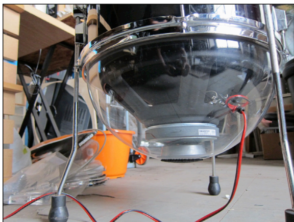
Figure 26 - 16" floor tom tonoscope with Celestion Truvox 1525 speaker mounted inside a 40cm acrylic dome
