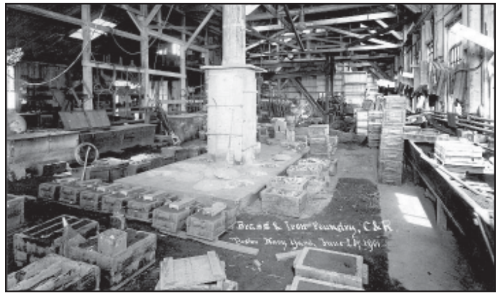
FOUNDRY, MOLD — A large number of molds can be seen in the foreground of this June 1901 view of the interior of the brass and iron foundry located in Building 16. These molds consist of frames containing wet sand formed around a pattern to create the cavity into which molten metal was poured. BOSTS-9279
