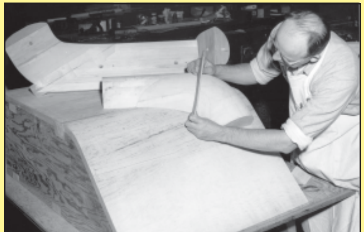
PATTERNMAKER — Patternmakers formed the wooden patterns from which molds were made for casting items in the Foundry. BOSTS-7755
