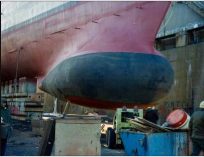
SONAR, KEEL BLOCKS — Most sonar units were installed in domes on the bow of the ship. This view shows the bow dome on USS Edward McDonnell (DE-1043) in Dry Dock 4 at the South Boston Annex on Jan. 9, 1973. Note the concrete keel block in the foreground with its wood “dunnage” at its side and the elevated keel blocks under the ship in the background.
