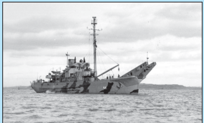
NET LAYING SHIP (AN) — USS Hoptree (AN-62, ex-YN-83) is seen on Dec. 2, 1944. Originally designated as Net Tender (YN), net laying ships (usually called net layers) serviced anti-submarine nets placed across harbors. Named for species of trees, the ships were based at Net Depots such as that located at the South Boston Annex. BOSTS-11434
