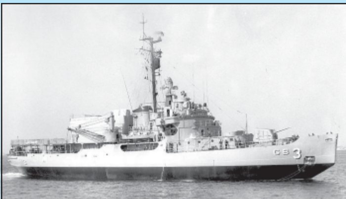
ICEBREAKER (AGB) — Icebreakers have reinforced hulls enabling them to break through ice fields. USS Atka (AGB-3) is seen in Mar. 1965 following the addition of a helicopter hanger at her stern. Built as USCG Southwind (WAG-280) and acquired by the Navy in 1950 after Lend-Lease service with the Soviet Navy, Atka and all other Navy icebreakers were transferred to the Coast Guard in 1966. BOSTS-10307
