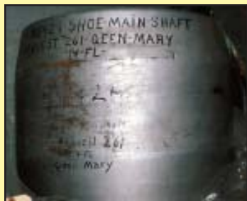
The collection includes a large sampling of patterns used to create everything from manhole covers for yard roadways to specialized components for ships. At left is a shoe pattern for the main shaft of HMS Queen Mary , while at right is one of hundreds of gear patterns. Brooke A. Childrey, BNHP
