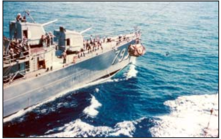
UNREP — Although underway replenishment is most often thought of in terms of refueling at sea, it also encompassed the transfer of ammunition and other supplies. Here, USS Cassin Young (DD-793) takes on fresh provisions from the storeship USS Aldebaran (AF-10) while operating in the Mediterranean in July or August 1959. Robert Norville
