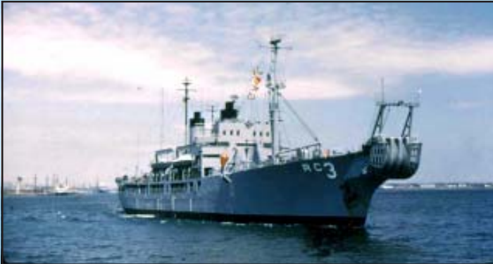
CABLE REPAIRING SHIP (ARC) — Cable repairing ships are easily recognized by the large sheaves on the bow used for laying and retrieving submarine communications cables. Although homeported at the Portsmouth Naval Shipyard, USS Aeolus (ARC-3), seen in May 1961, was a frequent customer of the Boston Naval Shipyard in the 1960s and early 1970s. BOSTS-16201
