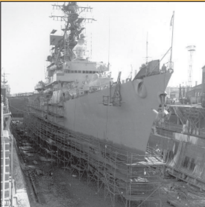
The transfer of Rommel to the German Navy did not end the vessel's association with the Charlestown Navy Yard. In late December 1970 the ship returned to Boston and entered Dry Dock 2 for work. Among the tasks performed was a repainting of her hull. This view taken on Jan. 13, 1971, shows the staging erected around the ship. BOSTS-14115
