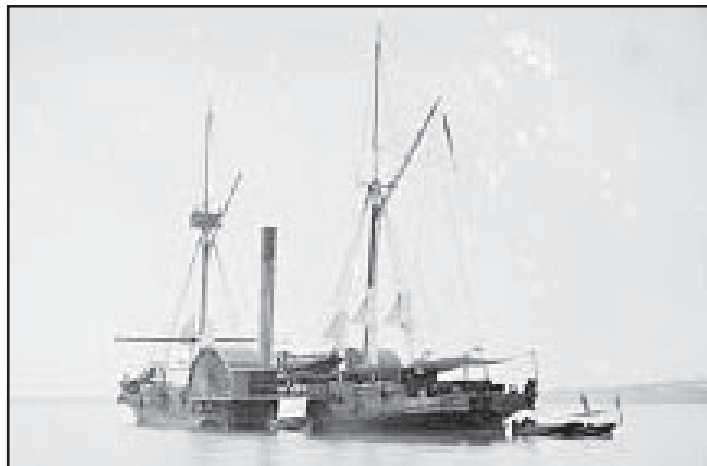
During the Civil War, the Navy Yard built five sidewheel double-end gunboats intended for service on coastal waters. The first of these ships, USS Maratanza , is seen here. BOSTS-11916
