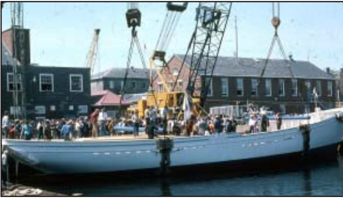
In the early 1980s, the New England Historic Seaport constructed the sail training schooner Spirit of Massachusetts alongside Dry Dock 2. Here, the vessel is lowered into the dock by a floating crane during her launching on Apr. 28, 1984. Warren Fuller, BNHP
