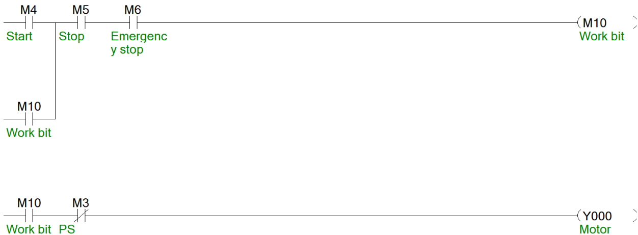
Figure 2-10. Control program solution.
