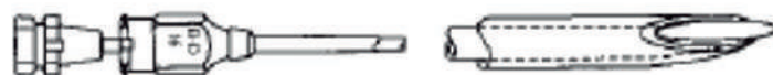
16 ga Tuohy-Flowers Needle 1950. Flowers dulled the sharp Tuohy needle tip and added a sharp stylet that would protrude past the needle tip to facilitate perforation of the skin. This design was prone to needle or stylet tip damage.
