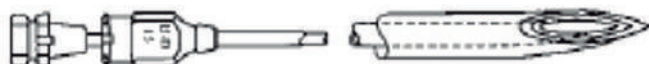
15 ga Huber Point Epidural Needle (Tuohy Needle) 1945. Tuohy can be credited with applying the Huber point (curved lip) design to the epidural needle and with adding a stylet. The needle tip was sharp as the intended application was continuous spinal anesthesia
