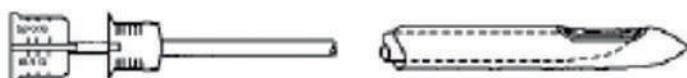
18.5 ga Special Sprotte Epidural Needle 1987. First "pencil-point" epidural needle to be used with a 23 ga epidural plastic catheter. Developed by Sprotte to minimize tissue trauma ("atraumatic needle")
