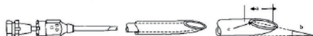
15 ga Hustead Epidural Needle 1954. (modified from the Tuohy needle) specified as a.) heel-to bevel distance < 27 mm b.) bevel angle of 12–15° and c.) a rounded heel to reduce the danger of trapping the catheter should it have to be withdrawn through the needle. A sharp 14 ga was used to break the skin. (first manufactured by Monoject 1964, 18 ga)
