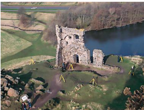
Figure 3 (left) Laser scanning at St Anthony's Chapel, Holyrood Park as part of the Rae Project in 2017 and (right) The 3D point cloud created. ©Historic Environment Scotland.
