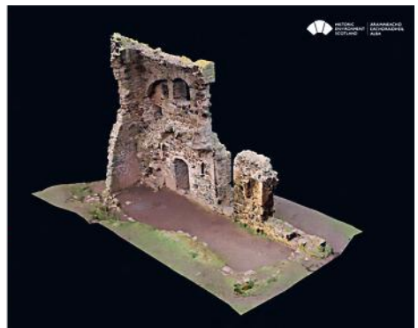
Figure 3 (left) Laser scanning at St Anthony's Chapel, Holyrood Park as part of the Rae Project in 2017 and (right) The 3D point cloud created. ©Historic Environment Scotland.
