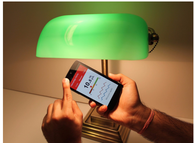
Figure 1: HemaApp is a smartphone application that noninvasively estimates blood hemoglobin concentration using a smartphone camera. Analysis of the color of the blood in a user's finger yields an estimate of the user's hemoglobin level. We evaluated the system using the smartphone's LED flash and incandescent light bulbs as illuminating sources.
