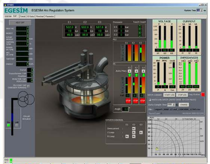
Arc Furnace SCADA Screen
