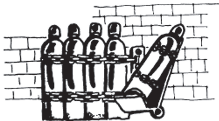
Secure gas cylinders adequately.
