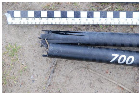
Fig. 2 Multi-fragment carbon fiber fishing rod fracture
