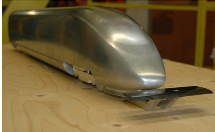
Figure 5: Wind tunnel model for the examination of fundamental aerodynamic and aeroacoustic properties of a front spoiler [22]
