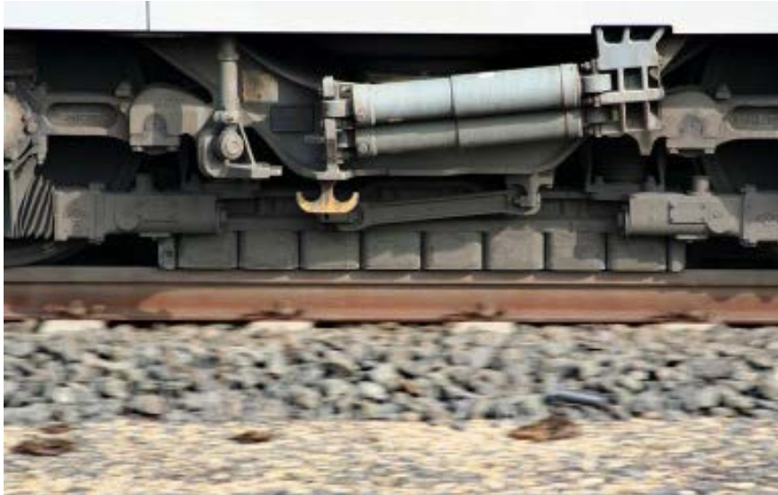
Figure 7: Linear eddy current brake of an ICE 3 in action [27]
