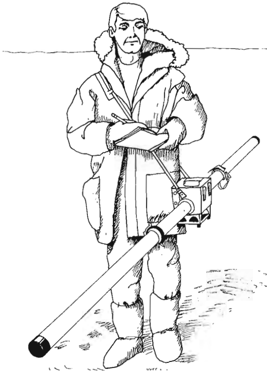
Figure 28.3. Schematic representation of the Geonics EM-31 system.
