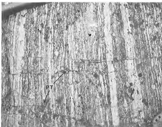
Figure 56.11. Mylonitic layering cut by late fractures and epidote veins. Locally generated pseudotachylyte (PT) zones are present. (GSC 203944-C)
