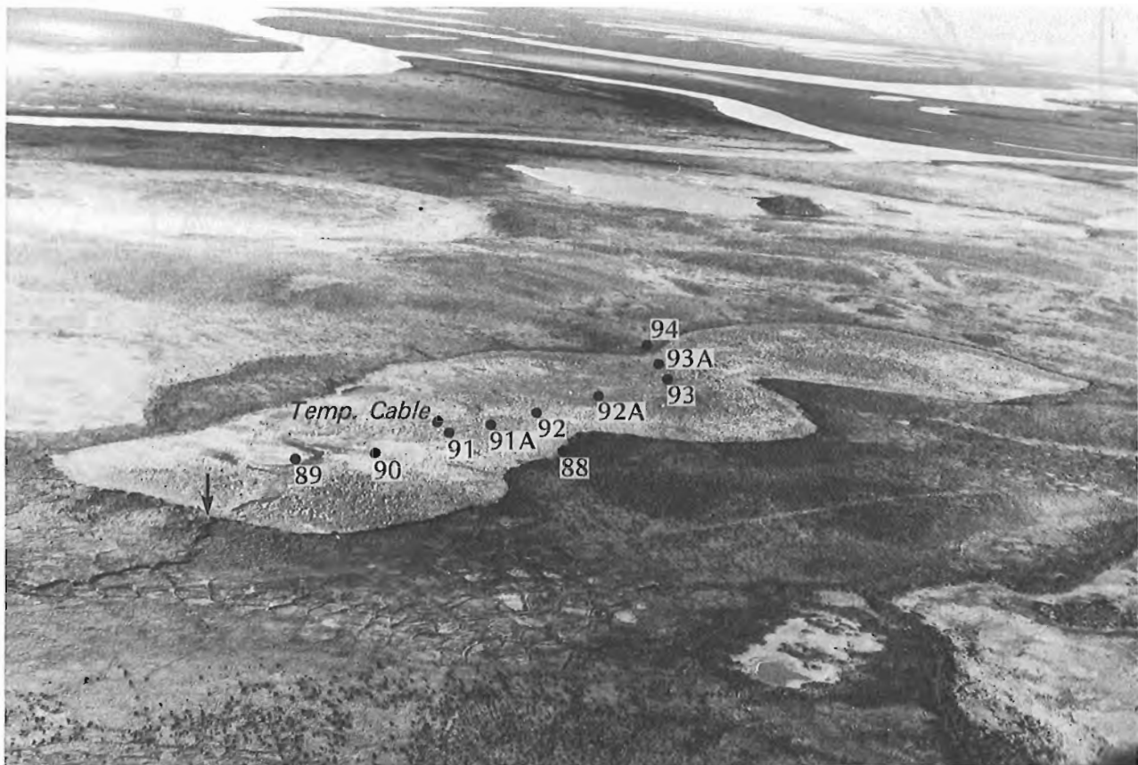
Figure 22.13. Lake 3 showing the locations of bench marks, temperature cable, and outlet (marked with an arrow). Photo taken in 1974.
