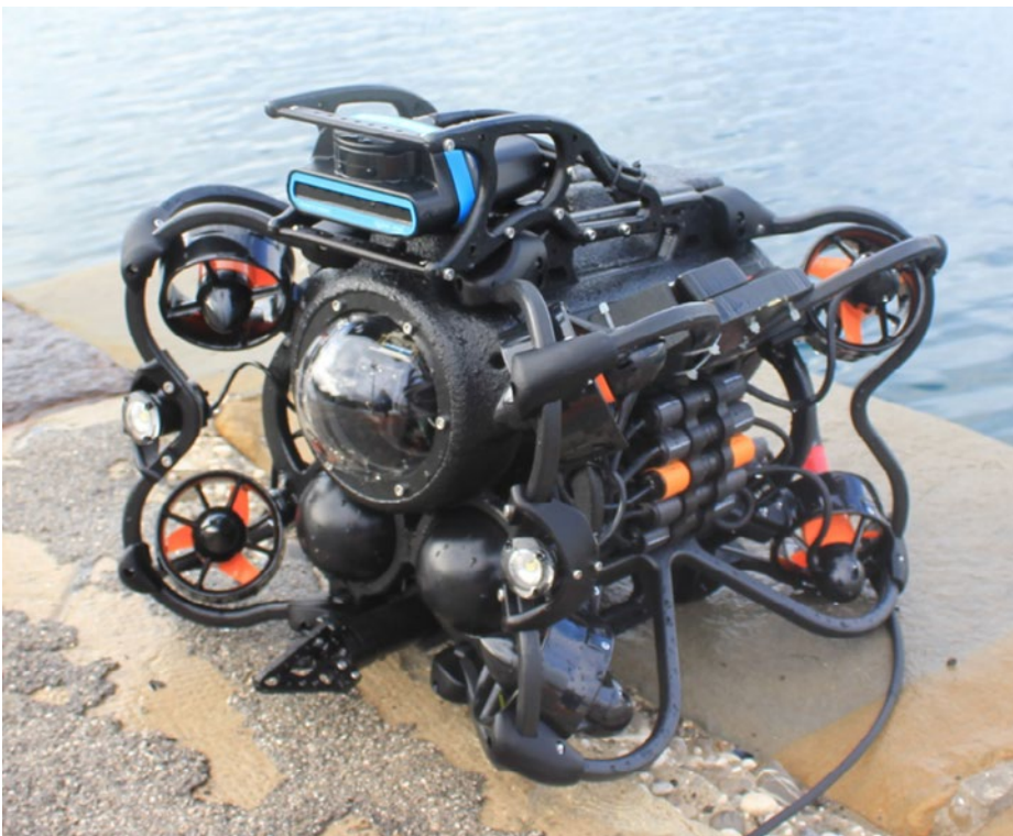
Figure 2. Power state of the art ROV driven by eight vectored trustor's and equipped with HD and 4K camera for seabed images and underwater video recording.
