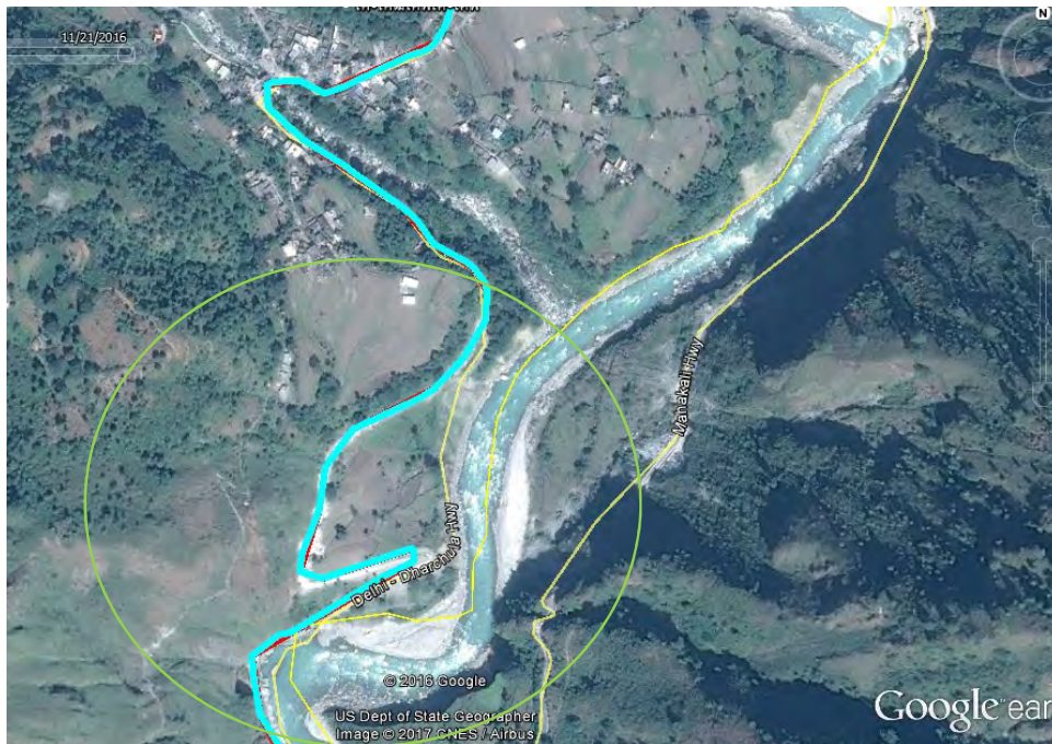
Figure 1 - With the Green circle – Kali meanders, the cyan colour represents the current alignment and the old alignment is in yellow coloured line. Similarly the meander near Baluwakot is almost a V pointing northwards, the main bazar is just abutting the river edge.
