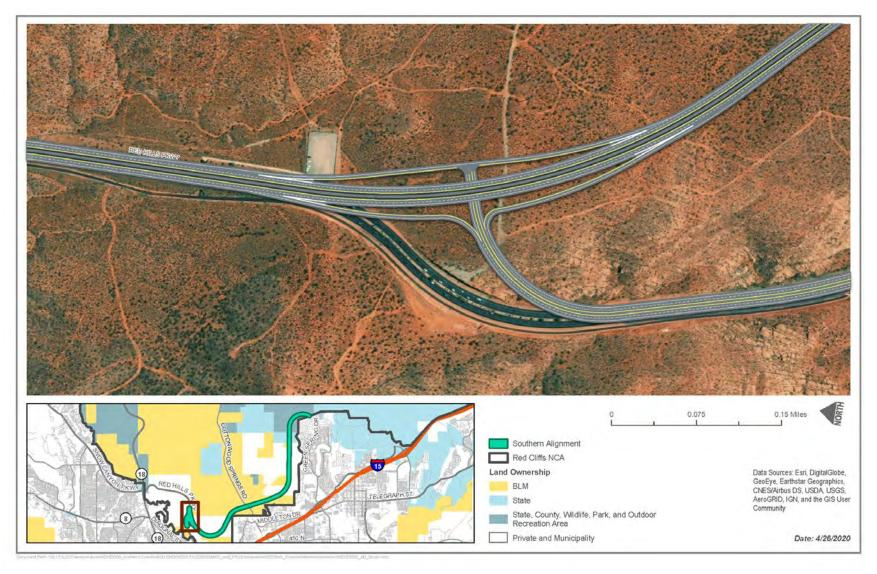
Figure 9a. Southern Alignment Plan View (1 of 11)
