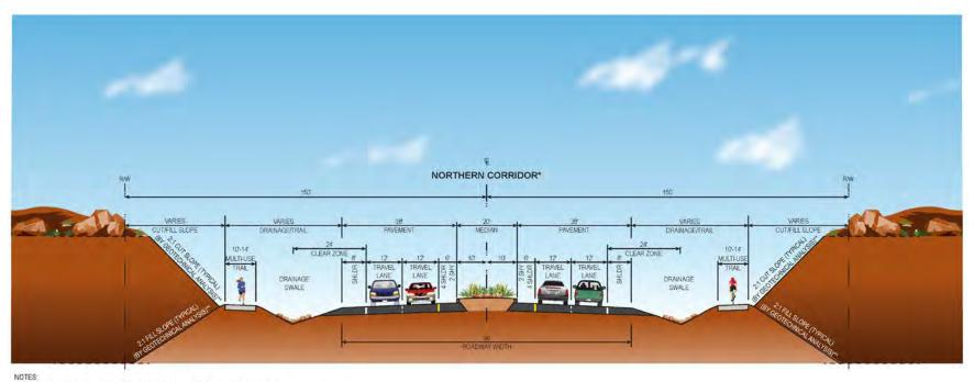
\*TOTAL ROW 300' - 500' DEPENDING ON SLOPE AND CONSTRUCTION REQUIREMENTS.
