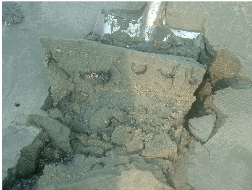
Fig. 5.1. Cross section of sediment from Prapas beach, April 2005. Fine sediment can be seen at the surface layer overlying coarser sediment (Photograph courtesy of G. Paterson)
