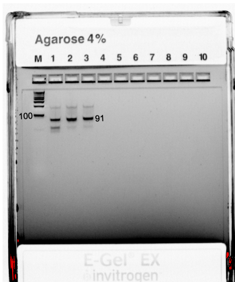
Figure 5. PCR product of barcode oligos ran on 4% agarose E-Gel. Primer-dimers seen in all lanes. Bottom of ladder bar corresponds to 100bp, barcode length: ~91bp.
