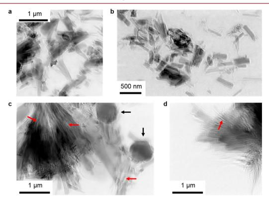
Figure 2. X-ray ptychographic images of  $CAH_{10}$  crystals: (a) and (b) before being subjected to heat curing; (c) and (d) after being stored at 60 ± 2 °C for 30 min. The black arrows indicate the  $C_3AH_6$  crystals, and the red arrows point to the clear morphological change in  $CAH_{10}$  prisms.
