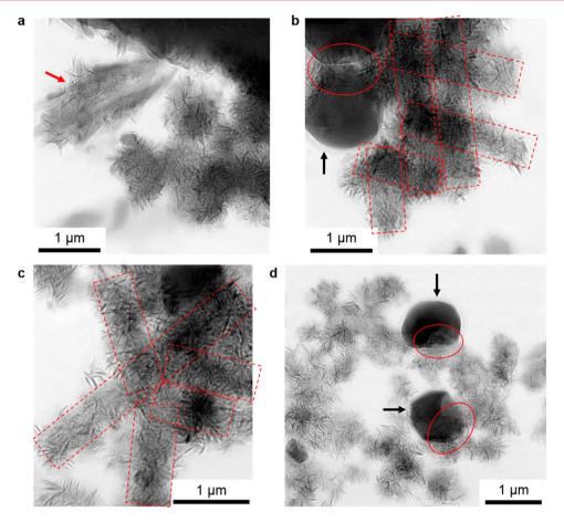
**Figure 3.** (a–d) X-ray ptychographic images of  $CAH_{10}$  stored at 60 ± 2 °C for 60 min. The black and red arrows indicate the  $C_3AH_6$  particles and a  $CAH_{10}$  prisms cluster in the middle of conversion, respectively. The red circles indicate the close contact between  $C_3AH_6$  crystals and the fiber morphology. The red dashed boxes indicate the prismatic contour of the fiber morphology.
