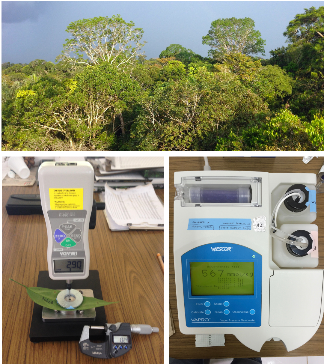
Figure S1.1: Top panel: Canopy view of Yasuní National Park near the 50ha plot. Lower left panel: Specific force to punch penetrometer (see Fig. S1.2 for baseplate schematics) and micrometer. Lower right panel: Osmometer used to estimate turgor loss point. Bottom pictures were taken at the Estación Científica Yasuní.
