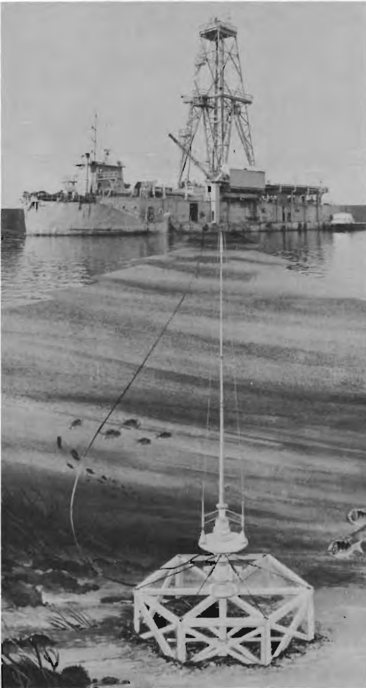
Figure 247. Schematic drawing of method developed by Continental, Union, Shell, and Superior Oil Companies for test drilling in water depths as great as 1500 feet. From Bauer, Crooke, and Stratton (1958). Modification of the method has permitted Global Marine Exploration Company to drill producing wells in a water depth of 350 feet and a total completion depth of 6250 feet.
