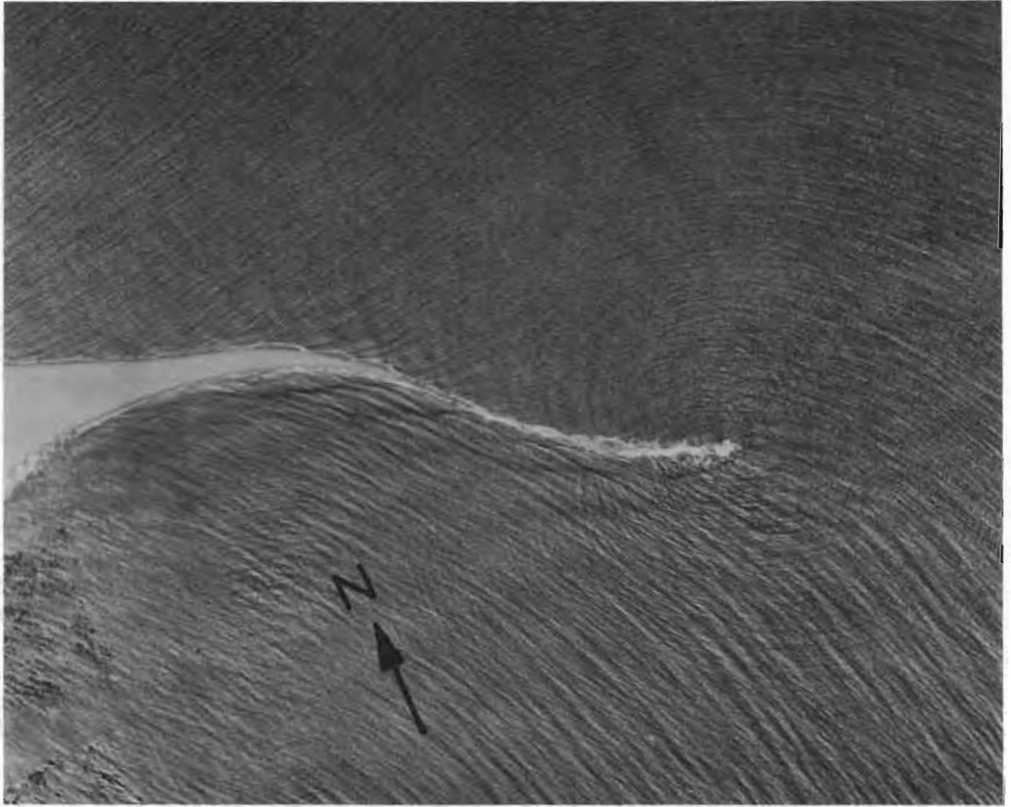
Figure 106. Wave refraction at San Nicolas Island. Swell from northwest is refracted around the island, meeting at a spit on the east side of the island and producing crossed wave crests beyond the end of the spit. Photograph by U. S. Geological Survey, courtesy of J. B. Schoellhamer.
