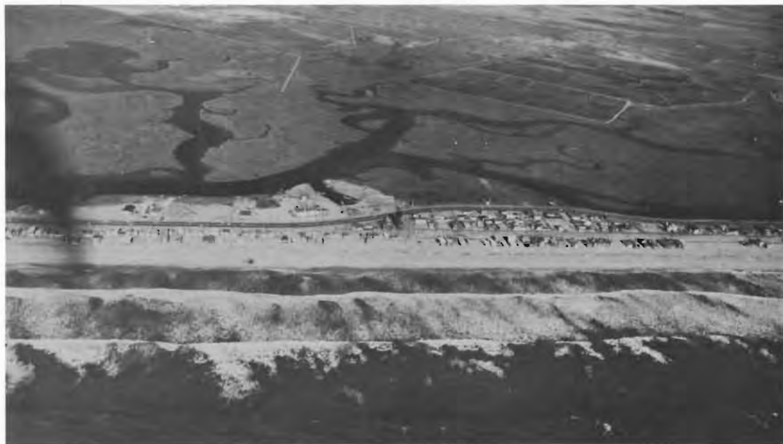
Figure 6. Seal Beach just west of breakwater. The wide offshore sand island provided quiet water for the accumulation of fine marsh sediments. Highly meandering tidal channels are typical of such marshes. Note the shortening of crest-to-crest spacing of waves as they approach the beach and enter progressively shallower water. Photographed by R. E. Stevenson in 1952.
