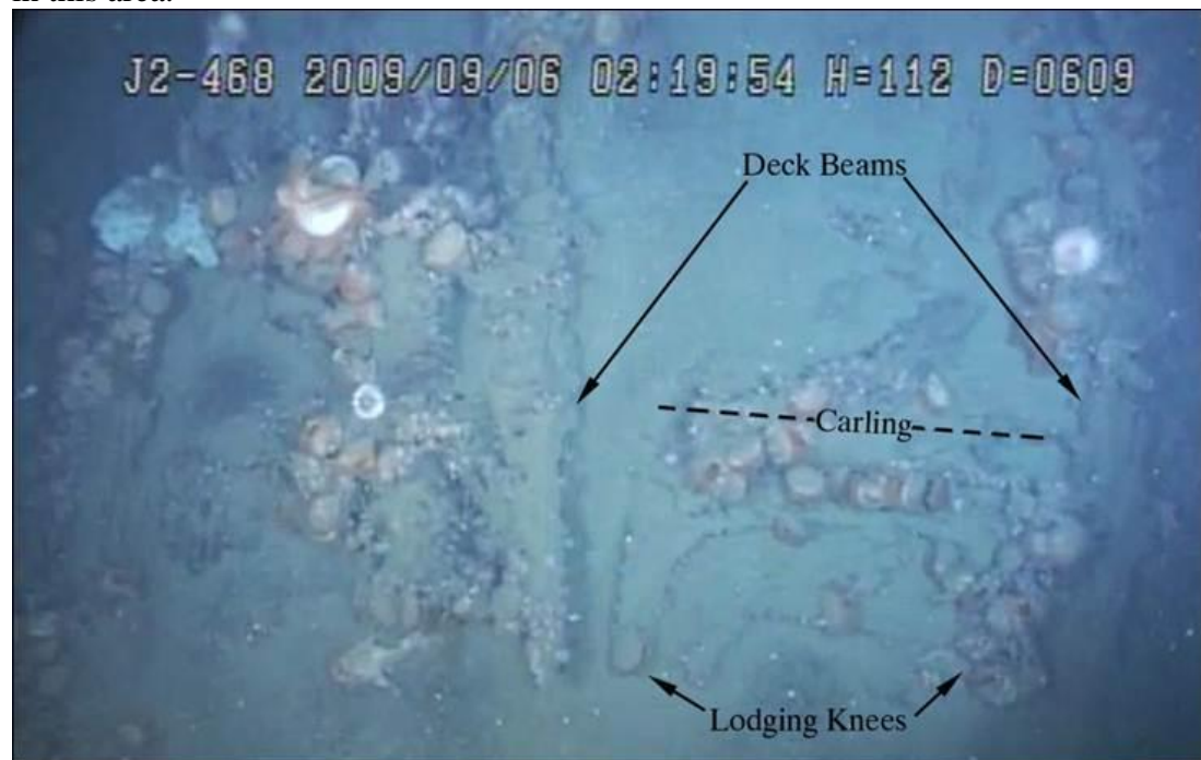
Figure 10-26. VK Wreck's deck structure from starboard view showing deck beams and lodging knees.
