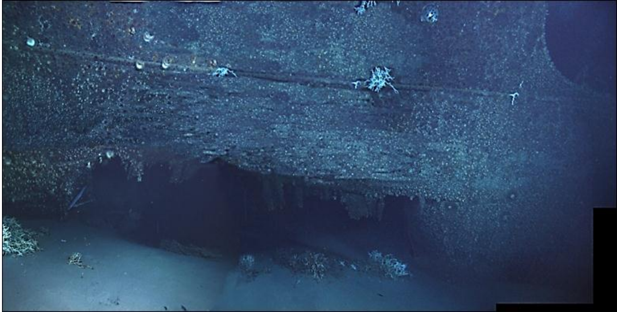
Figure 10-144. Hole from the second torpedo.
