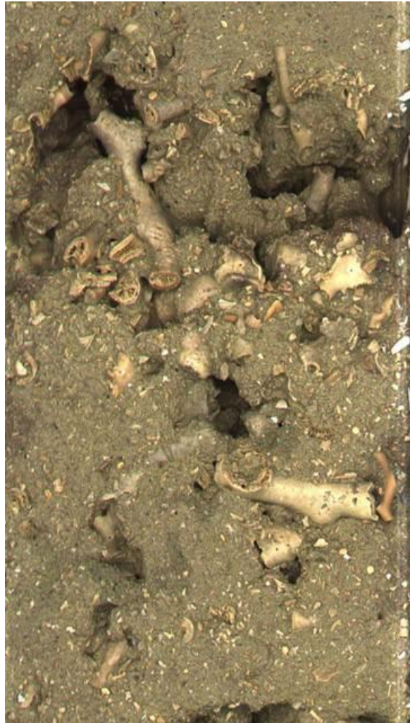
Figure 9-8. This photograph is a close-up of the middle of Section 4 of the Mound Crest 2 JPC illustrated in the previous figure. Note the densely packed coral “sticks” and smaller fragments. The matrix sediment is rich in clay minerals and calcareous microfossil tests. The width of the core photograph is ~ 12 cm (5 in).
