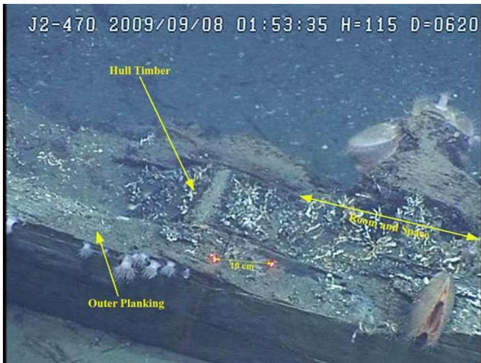
Figure 10-85. ROV video capture image showing the Ewing Bank Wreck's outer hull planking, hull framing, and interior ceiling planking.
