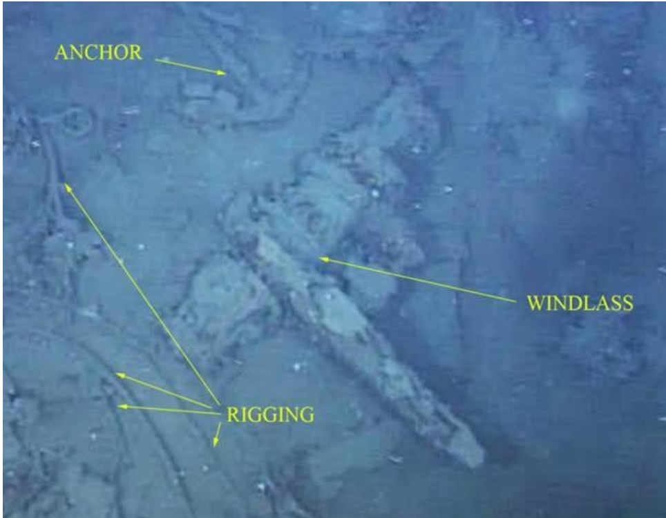
Figure 10-43. Overhead view of the over-turned windlass on 7,000 Foot Wreck, bow is toward upper left corner of image.
