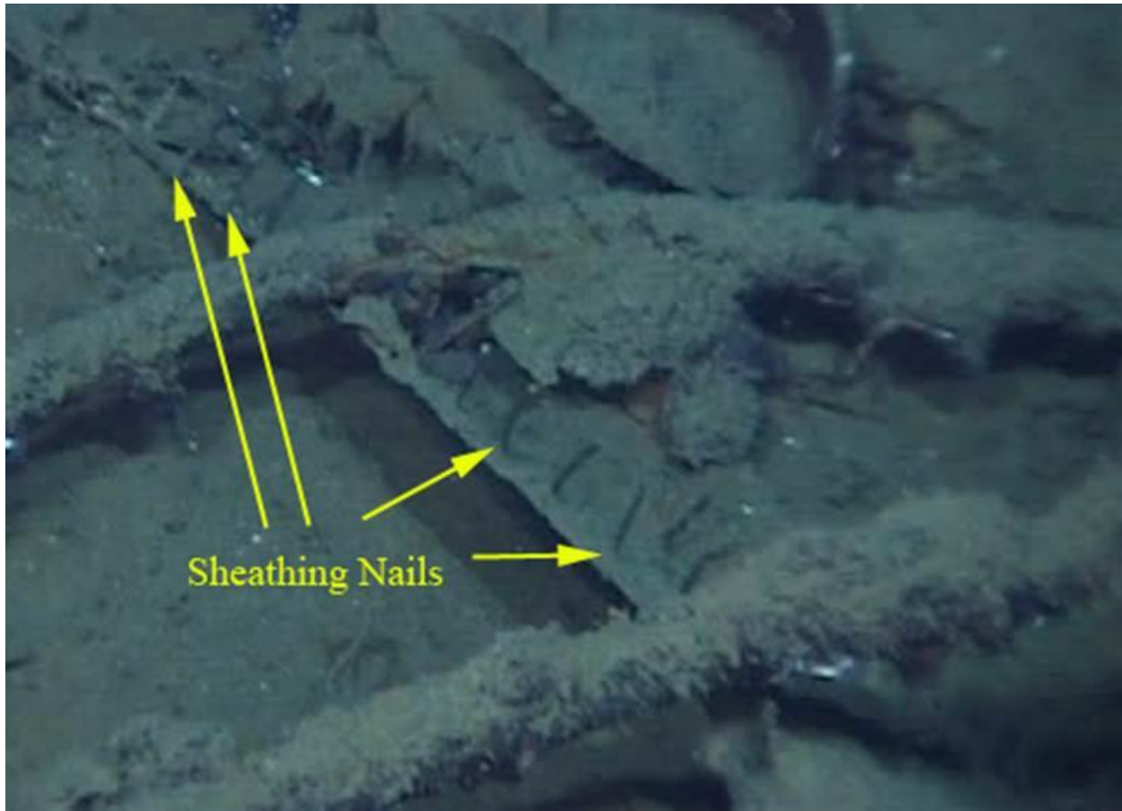
Figure 10-52. Close-up of a section of sheathing with sheathing nails intact in the 7,000 Foot Wreck.
