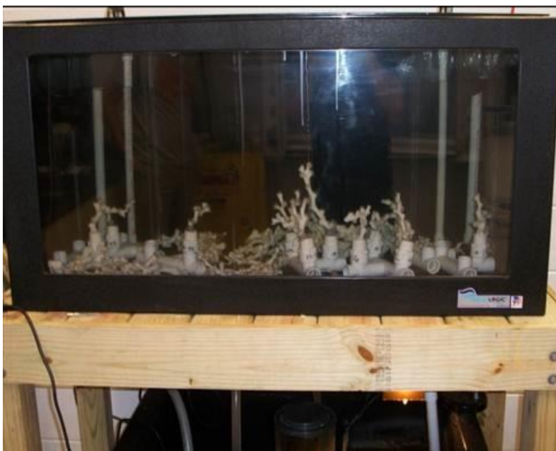
Figure 7-1. Representative example of maintenance aquarium setup. The upper aquarium is the display tank and held the corals and associates. Below the aquarium is the sump tank and requisite filtration compartments.
