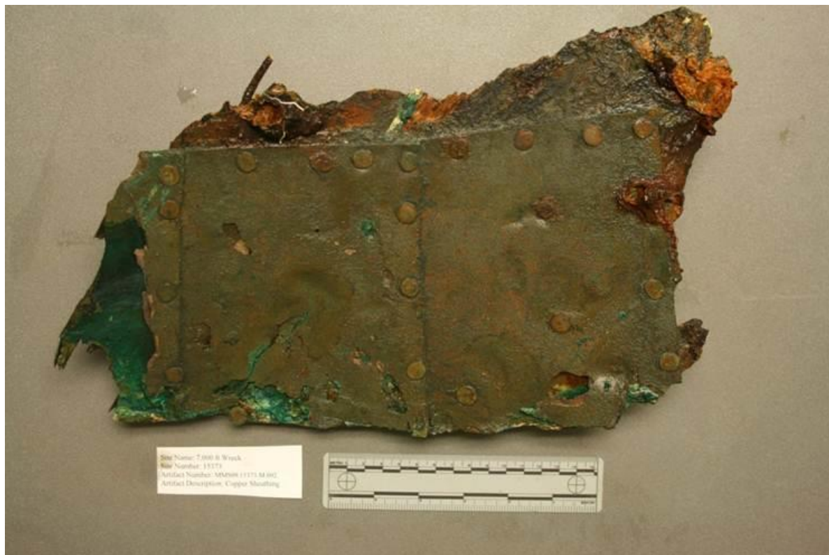
Figure 10-68. Cuprous metal sheathing and wood recovered from the 7,000 Foot Wreck.
