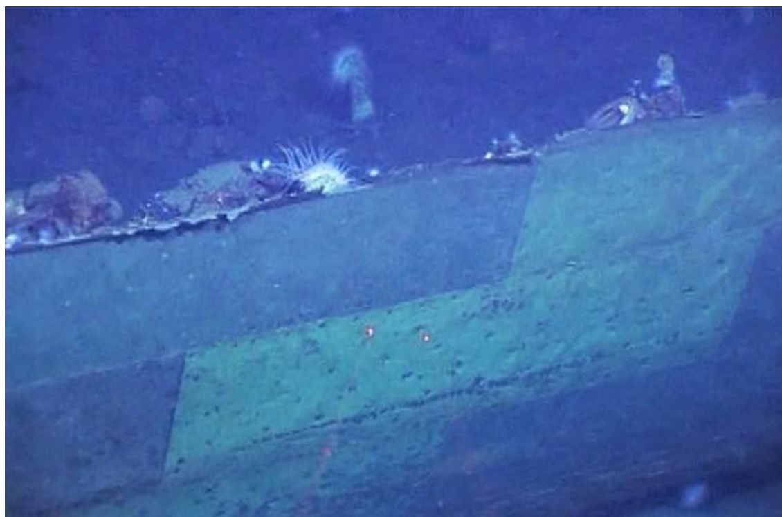
Figure 10-96. ROV video capture image showing Muntz metal copper sheathing and possible repair areas on the Ewing Bank Wreck's starboard hull.
