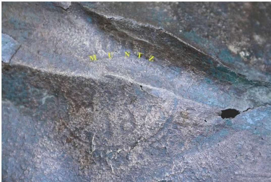
Figure 10-113. Close-up of Muntz Metal maker's stamp on sheathing sample recovered from Ewing Bank Wreck (University of West Florida).
