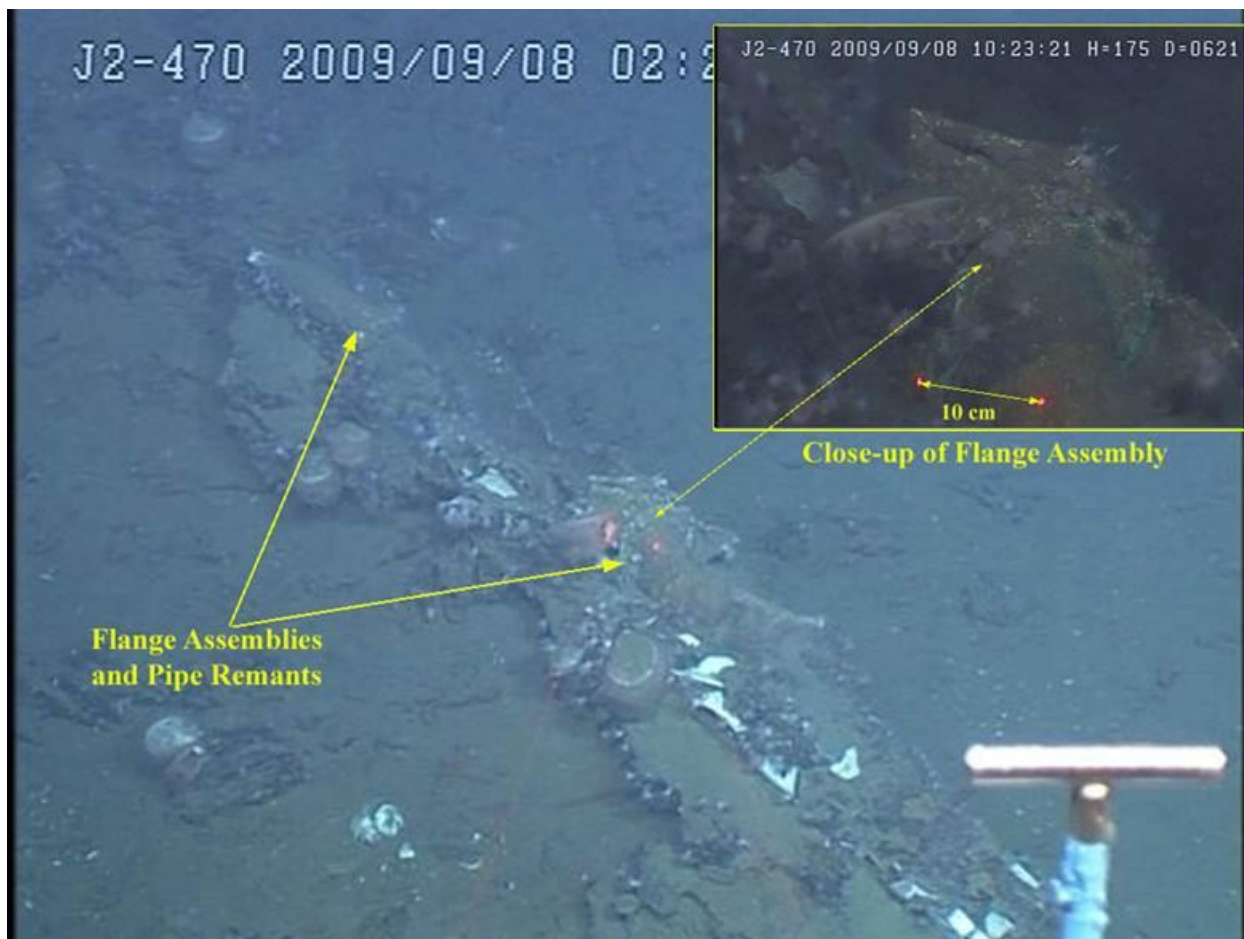
Figure 10-103. ROV video capture image of flange assemblies and pipe remnants on the Ewing Bank Wreck's port stern.
