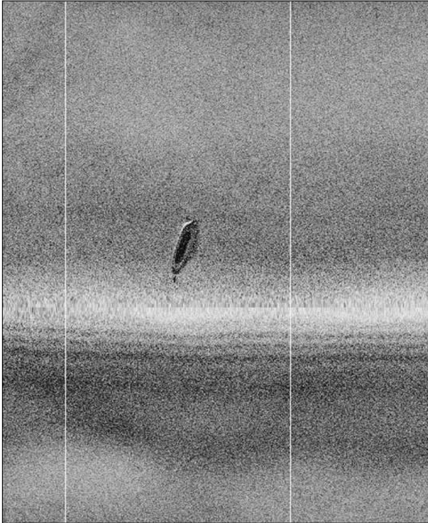
Figure 10-70. A 2006 210p- kHz side scan sonar image of the Ewing Bank Wreck (ATP Oil and Gas).
