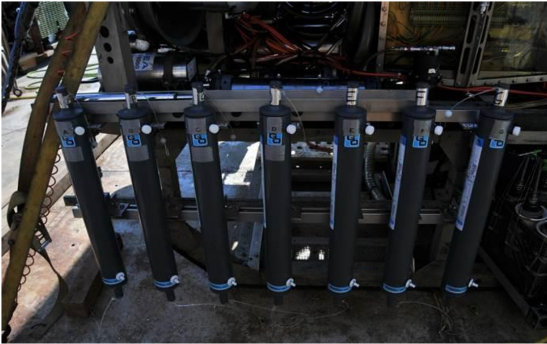
Figure 3-1. Seven Niskin bottle array fitted to ROV Jason during the 2010 Lophelia II cruise.
