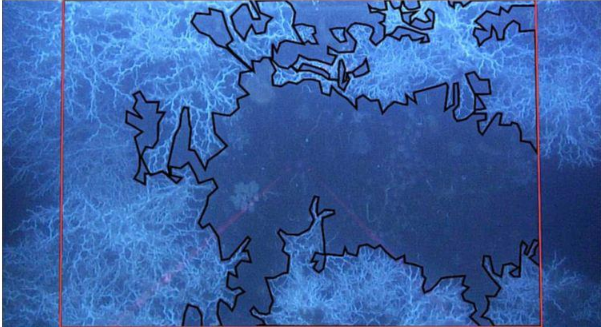
Figure 8-16. Example of screen shot used for percent coverage analysis. Structure G at 304 m with 57% of the structure covered with L. pertusa . The structure is outlined in red and the L. pertusa covering the platform surface are outlined in black.
