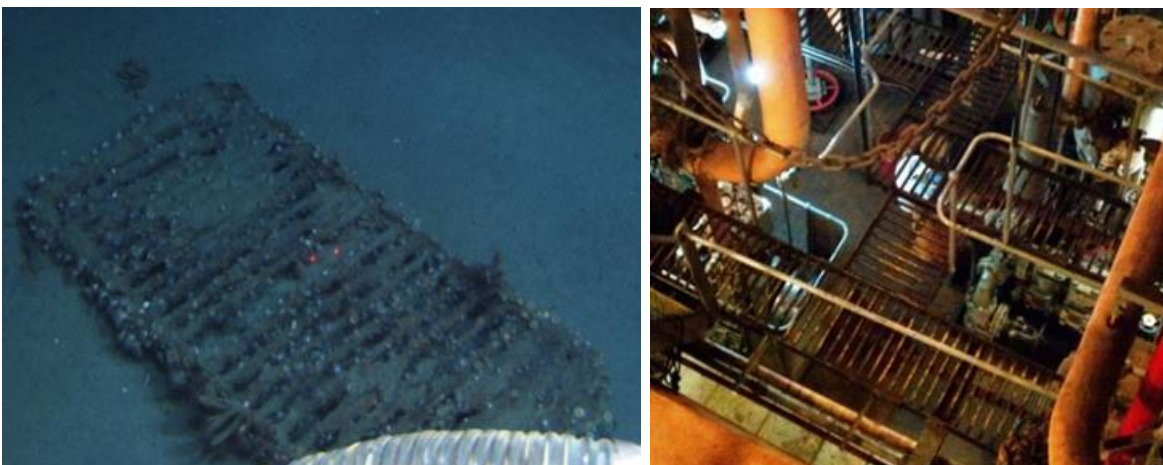
Figure 10-137. Deck grating from Gulfoil (left) and deck grating from Jeremiah O'Brien (right) ( Jason II ROV camera; William M. Briggs, 1012).
