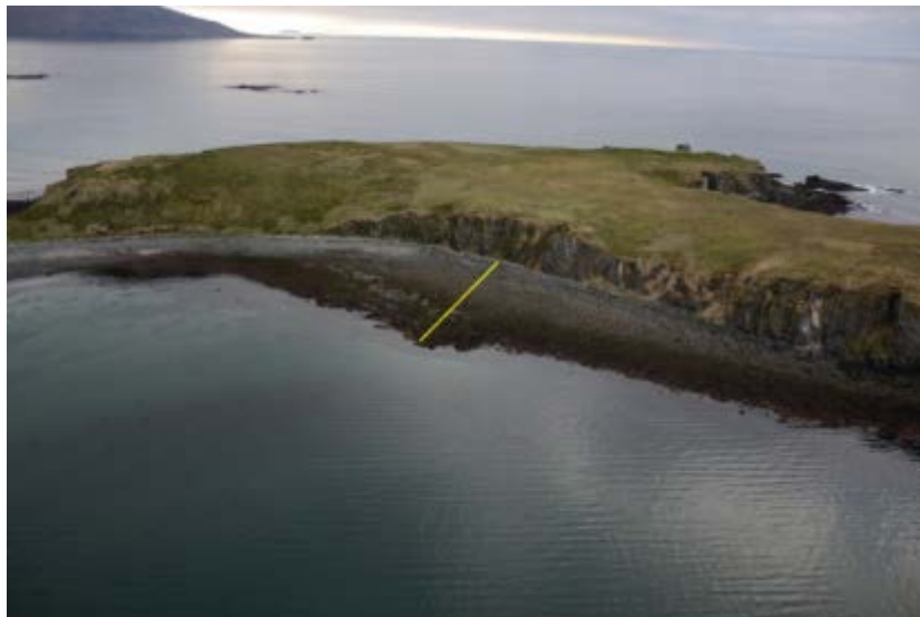
Figure D-71. Aerial photo of site AKP_16_024 from ShoreZone aerial survey May 7, 2016. Yellow line shows location of transect where site profile was measured.
