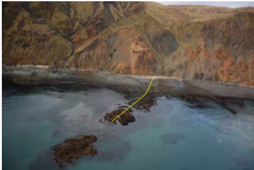
Figure D-20. Aerial photo of site AKP_16_007 from ShoreZone aerial survey May 7, 2016. Yellow line shows location of transect where site profile was measured.
