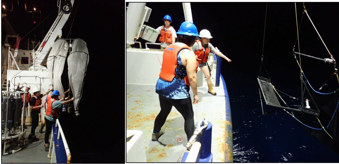
Figure 17. Bongo net (left) being deployed for a vertical cast to a depth of 100 m during the EN626 cruise
