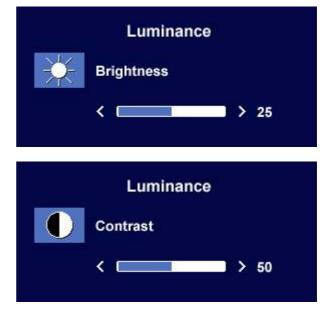
Press the  $\blacktriangleleft$  or  $\blacktriangleright$  keys to adjust the degree of **Contrast**.
