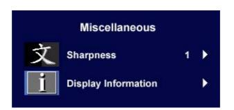
Press the  $\blacktriangleleft$  or  $\blacktriangleright$  keys to adjust the degree of Sharpness.
