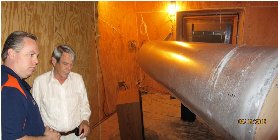
Figure 98: Experimental setup of the 24 inch diameter steel cylinder.
