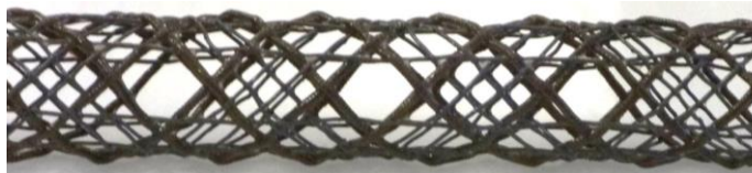
Figure 70: Manufacturing of an open architecture composite tube. 70
