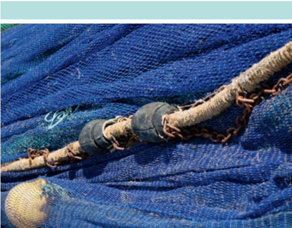
Use of rollers and chain on the sea anchor of a trawling net, in the province of Huelva. © OCEANA/ M. Cornax
