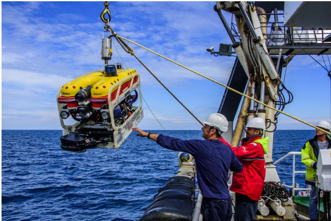
Figure 11. ROV operator and deckhand launching the ROV into the water. © OCEANA/ Juan Cuetos
