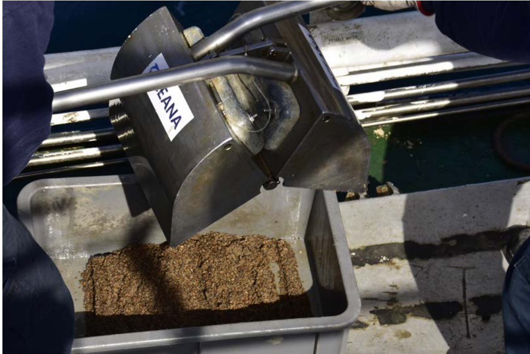
Figure 13. Van Veen grab sampler collecting a sample of coarse sand. © OCEANA/ Carlos Minguell
