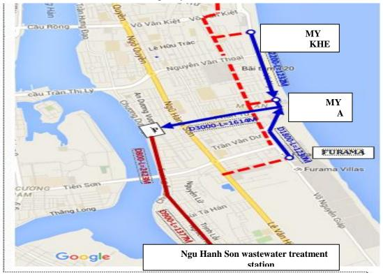
Figure 1-9: Solution for wastewater treatment at My An and My Khe outlet
