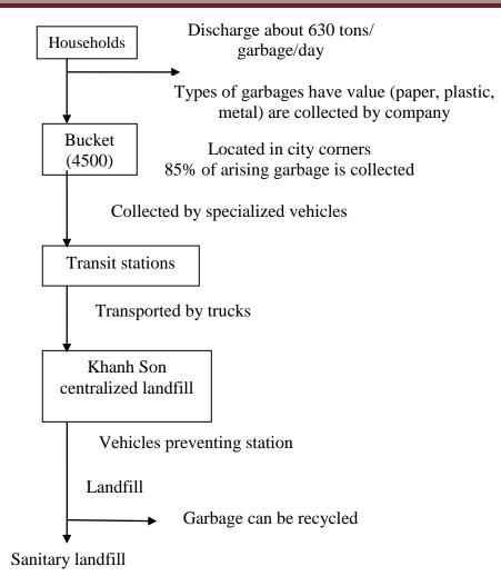
Figure 2-8: Solid waste management system in Da Nang city
