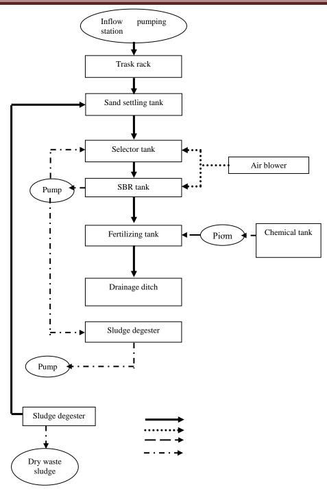
Figure 1-16: Diagram of SBR wastewater treatment technology
